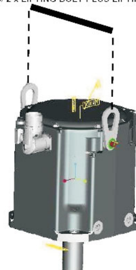
B3/ 2 x LIFTING BOLT PLUS LIFTING BEAM
