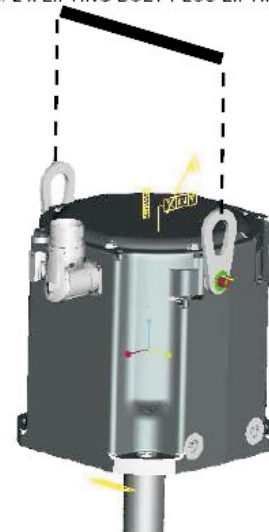
B3/ 2 x LIFTING BOLT PLUS LIFTING BEAM
