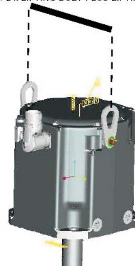
B3/ 2 x LIFTING BOLT PLUS LIFTING BEAM
