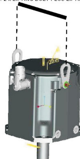
B3/ 2 x LIFTING BOLT PLUS LIFTING BEAM
