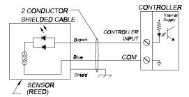
**Note:** The <u>black</u> wire in *Quick Disconnect* cables is not used with any version of the PSR (Reed) sensor. In the above drawing, only the blue wire, brown wire, and shield are connected.
