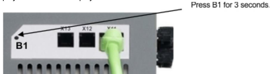
4. When the display blinks with the set rotary switch setting stop pushing B1 and wait until the blinking stops. During that time the parameter FBUS.PARAM01 is set to the new value and all parameters are stored to the non volatile memory. The new setting will be taken with the next power-up of the drive.
