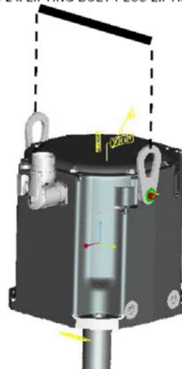
B3/ 2 x LIFTING BOLT PLUS LIFTING BEAM
