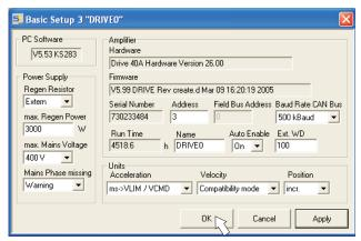
Regen Resistor: Select "external" regen resistor
