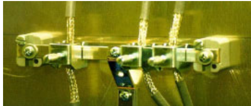
Example of a complete shield connection.
