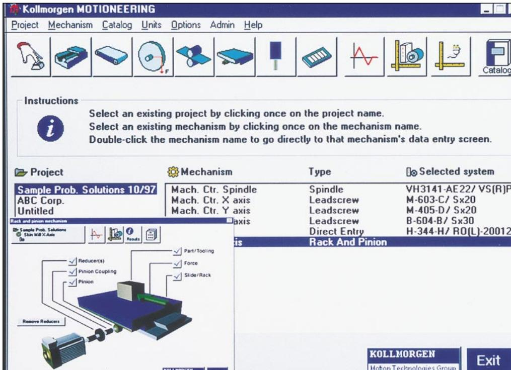
Numerous software packages are available to help take the drudgery out of defining motion profiles and selecting the optimum servomotor, amplifier, and power supply. Motioneering from Kollmorgen is such a tool on CD-ROM that runs in Windows. It calculates shunt regeneration for multiple axes, and simulates foldback circuits to ensure that the motor and amplifier combination considers the amplifier's time constant.
