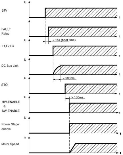
Fault F602 occurs when STO (=> p. 53) does not have current when HW enable becomes active.
