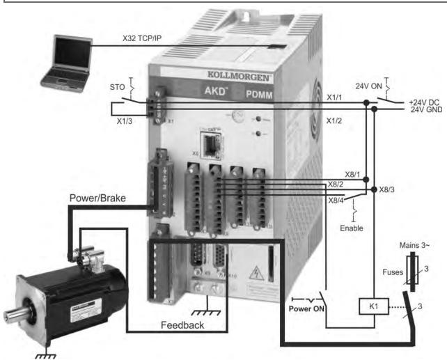
When connecting the AKD PDMM directly to a PC, static IP addressing (not 0) is recommended.
