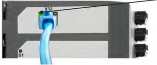
LED is green if drive is connected through a network device.
