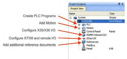
All drives, including the drive in the AKD PDMM itself, and the Remote I/O can be configured by the KAS IDE. Add the drives to the project: click on the EtherCAT item and scan for devices (1).
