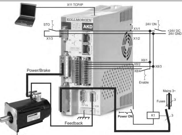
When connecting the AKD directly to a PC, static IP addressing (not 00) is recommended.
