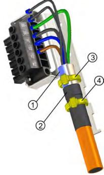
Strip the external cable sheath to a length of approx. 120 mm, taking care not to damage the braided shield. Push the braided shield (1) back over the cable and secure with a rubber sleeve (2) or shrink sleeve.
