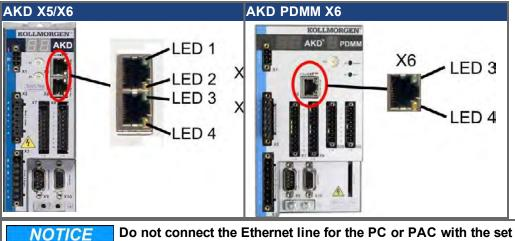
Do not connect the Ethernet line for the PC or PAC with the set up software to the motion bus interface X5/X6.
