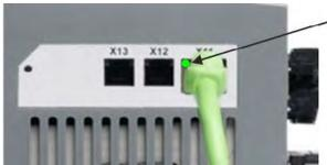
LED is green if drive is connected through a network device.
