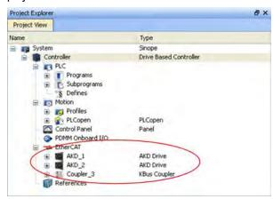
To communicate directly with a drive without running a project click on the EtherCAT item in the project tree. Click on the drive in the project tree to configure (1), then click on the **Online Configuration** button (2):
