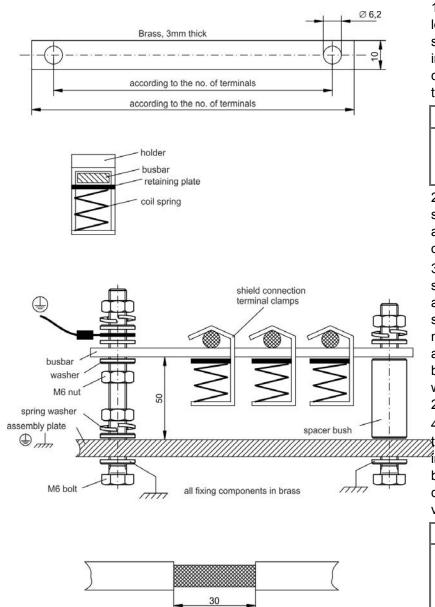
1. Cut a busbar of the required length from a brass rail (crosssection 10 x 3 mm) and drill holes in it as indicated. All shield clamps required must fit between the drill holes.
