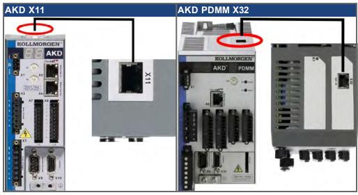
Connect the service interface (X11 or X32) of the drive to an Ethernet interface on the PC directly or via a network hub/switch, while the supply to the equipment is switched off. Use standard Cat. 5 Ethernet cables for connection (in some cases crossover cables will also work).
