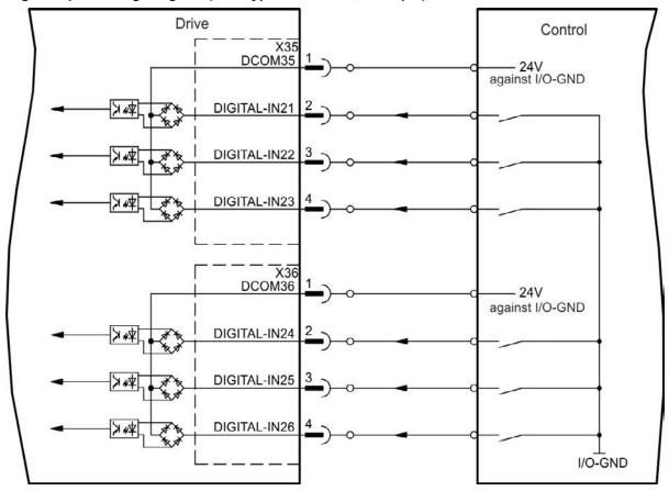
Digital Input Wiring Diagram (Sink type connection, example)
