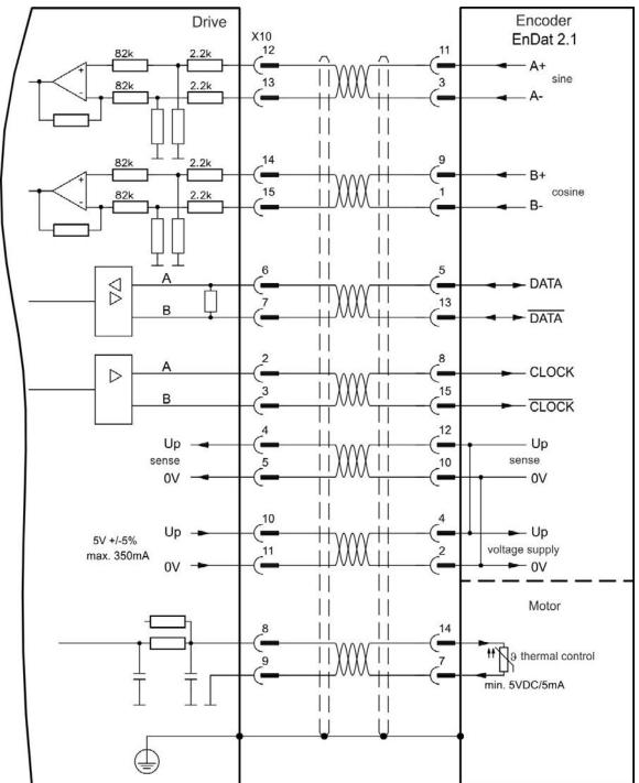
The pin assignment shown on the encoder side relates to Kollmorgen™ motors.
