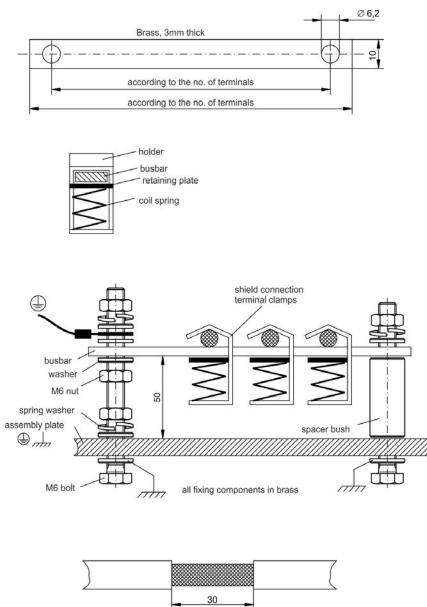
1. Cut a busbar of the required length from a brass rail (crosssection  $10 \times 3$  mm) and drill holes in it as indicated. All shield clamps required must fit between the drill holes.
