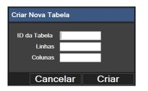
Enter the table ID, the number of rows, the number of columns, and then click on the "Create" button. A table will be created with the entered properties. All fields in this new table will have the value "0". The file name of this table will be the number entered in the "ID" field and with the extension ".TAB".
