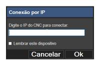
Enter the IP of the CNC you want to connect to and click the "OK" button Once this is done, the CNC should appear in the list.
