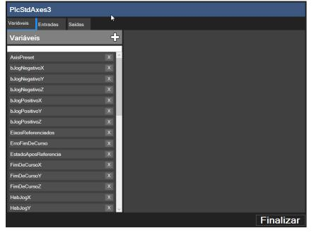
On this screen we can add, edit and remove variables that will be used in the PLC program. On this screen we can also define the variables for digital inputs and outputs.
