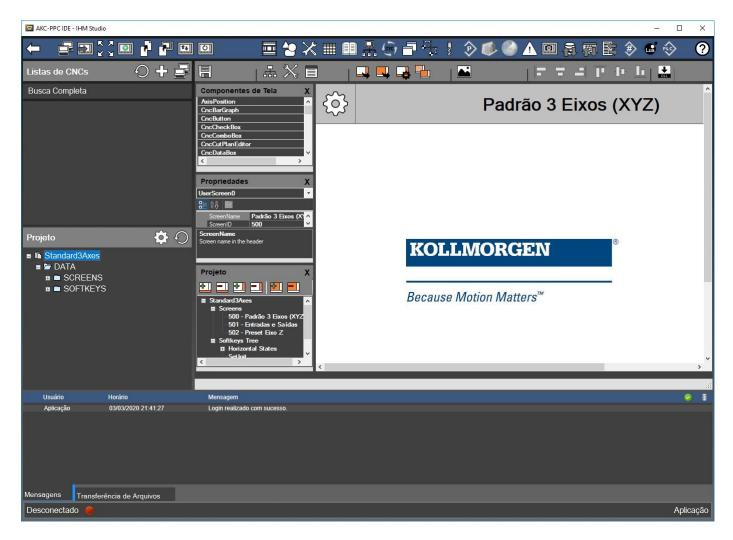
On the left side of this screen, at the top is the list of CNCs to connect to, and below is the structure of the "Project" containing the folders and files related to the HMI Studio. On the right side we have the HMI Studio editor.
