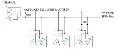
Note: A termination resistor must be inserted in the first and last driver of the circuit.
