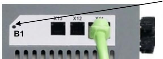
The seven segment display shows **Cn** during the process of changing DRV.TYPE to CAN.
