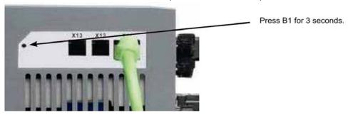
The seven segment display shows **En** during the process of changing DRV.TYPE to EtherCAT. **Do not switch off the 24[V] power supply while the seven segment shows En!**
