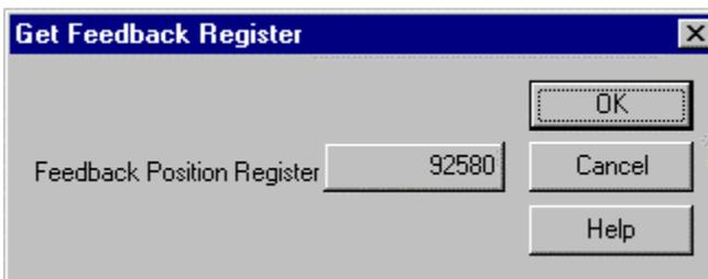
**Example:** If the motor utilizes a 1000 line encoder there are 4000 pulses per revolution of the motor. If the Feedback Register was 92580 counts the corresponding motor position is 23.145 revs.
