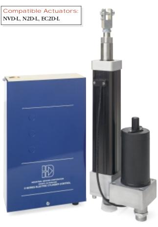
The D2500B Series is an analog position control which accepts an analog voltage or current command input and translates the signal into a proportional linear displacement. The control is used with electric cylinders containing a linear potentiometer (-L) option. Feedback from the linear potentiometer is proportional to distance. The control compares this feedback to the scaled command input, providing a closed loop linear positioning system.
