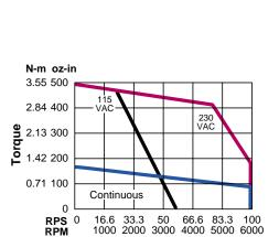
Continuous duty region (230/115 VAC) max RMS torque over any 10-minute interval]
