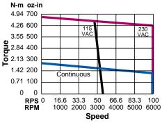
Continuous duty region (230/115 VAC) [max RMS torque over any 10-minute interval]
