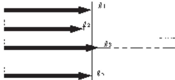
$$\text{Positioning Repeatability} = \pm 1/2 \{(\text{Maximum value of } \ell \text{ } n) - \text{Minimum value of } \ell \text{ } n\}$$
