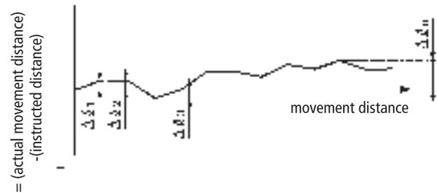
$$\text{Positioning Accuracy} = (\Delta \ell \text{ } n)_{\text{max}}$$
