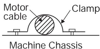
**Note:** Ground shield to machine chassis with a metal clamp providing a 360 degree termination cable.
