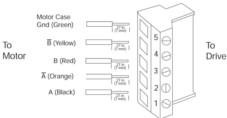
**Note:** The colors in the diagram follow the Pacific Scientific stepper motor cable color code.
