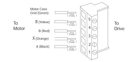
**Note:** *The colors in the diagram follow the Pacific Scientific stepper motor cable color code.*
