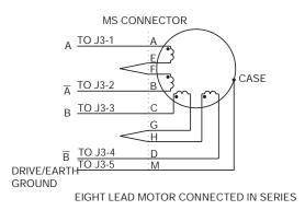
Power Max motor connections The figure below shows the connections required between the 6415 and Pacific Scientific Power Max Motors. Power Max motors have an eight pin connector and can be configured with either parallel or series windings.
