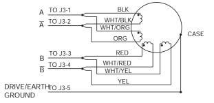
EIGHT LEAD MOTOR CONNECTED IN PARALLEL
