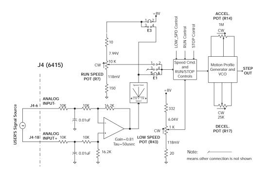
External analog input with internal RUN SPEED pot
