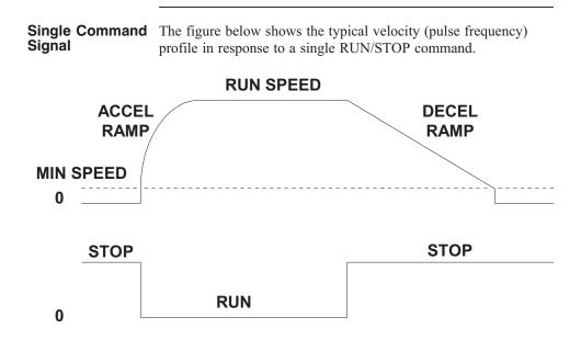
Acceleration rate is non-linear resulting in an exponential velocity ramp. Deceleration rate is constant, resulting in a linear velocity ramp. Accel Ramp Potentiometer (R14) and Decel Ramp Potentiometer (R17) adjust the time for acceleration and deceleration. With fixed accel potentiometer and step size settings, the acceleration rate is a function of speed control inputs. For example, increasing the run speed command by a factor of two will result in twice the acceleration rate.
