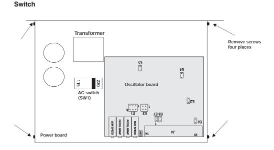
**Note:** *The AC Switch is preset at the factory in the 230 Vac position.*
