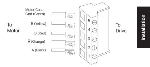
**Note:** *The colors in the diagram follow the Pacific Scientific stepper motor cable color code.*
