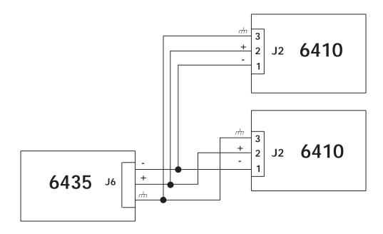
**Note:** If the 6435 is powering additional 6410s with J6, a total of 1000  $\mu$ f (maximum) 100 Vdc aluminum electrolytic capacitor, rated for 2A ripple current or greater (a) 10 KHz and 105°C, must be installed at the 6410 (as close to the 6410 as possible) if the cable length is over 3 feet. **DO NOT** exceed 1000  $\mu$ f total on J6 external connector.
