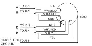
EIGHT LEAD MOTOR CONNECTED IN PARALLEL
