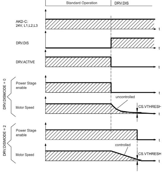
If velocity drops below threshold CS.VTHRESH or timeout occurs brake is applied.
