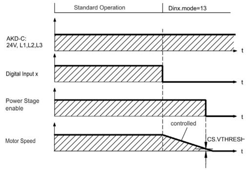
If velocity drops below threshold CS.VTHRESH or timeout occurs brake is applied.
