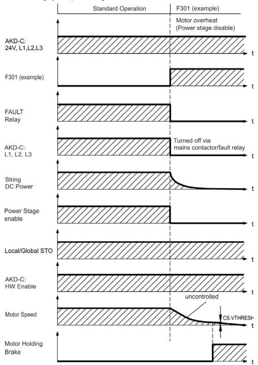
If velocity drops below threshold *CS.VTHRESH* or timeout occurs the motor holding brake is applied. Set parameter MOTOR.BRAKEIMM to 1 with vertical axes, to apply the motor holding brake immediately after faults.
