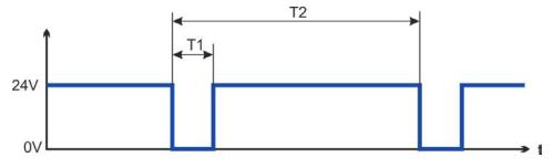
Test pulses with T1 < 300 µs and T2 > 200 ms will not have any influence to the safety relevant STO function. Test pulses, which are outside of this specification, will switch the STO function, but will not create a dangerous situation.
