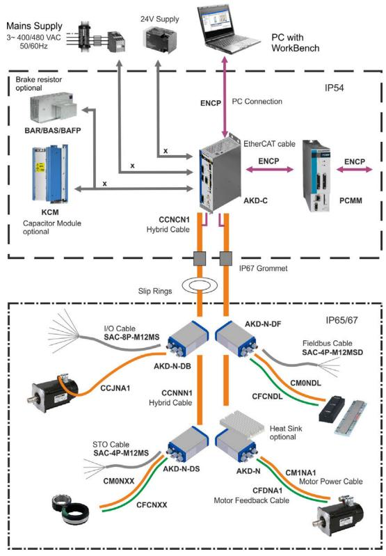
All components inside the borders are supplied by Kollmorgen with the exception of cables signed with "x". These cables are not supplied by Kollmorgen, you should use cables or wires according to EN 60204.
