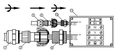
Remove the outer covering over length B, without damaging the shielding braid. Shorten the shielding braid to length A.
