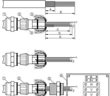
Remove the outer covering over length B, without damaging the shielding braid. Shorten the shielding braid to length A.
