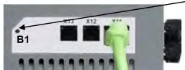
4. When the display blinks with the set rotary switch setting stop pushing B1 and wait until the blinking stops. During that time the parameter FBUS.PARAM01 is set to the new value and all parameters are stored to the non volatile memory. The new setting will be taken with the next power-up of the drive.
