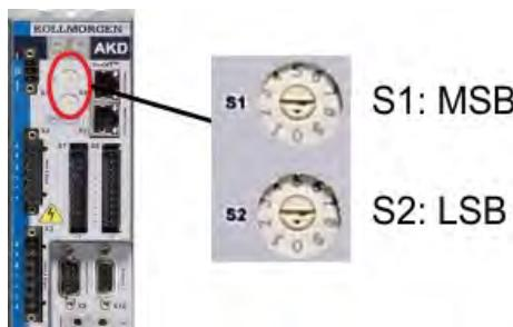
The rotary switches on the front of the AKD (S1&S2) correspond to the CAN node address. The S1&S2 switches also correspond to the IP address setting of the drive. Both CAN and IP network address schemes have to be configured to account for this dependence if both TCP/IP and CAN networks are running at the same time in an application. Example:
