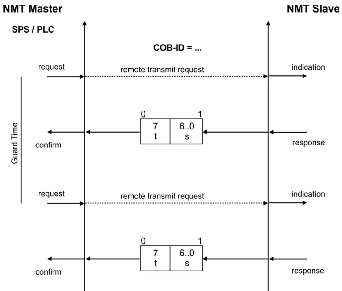
Node guarding is carried out by the Master through RTR telegrams with the COB-ID 700h + slave node address.
