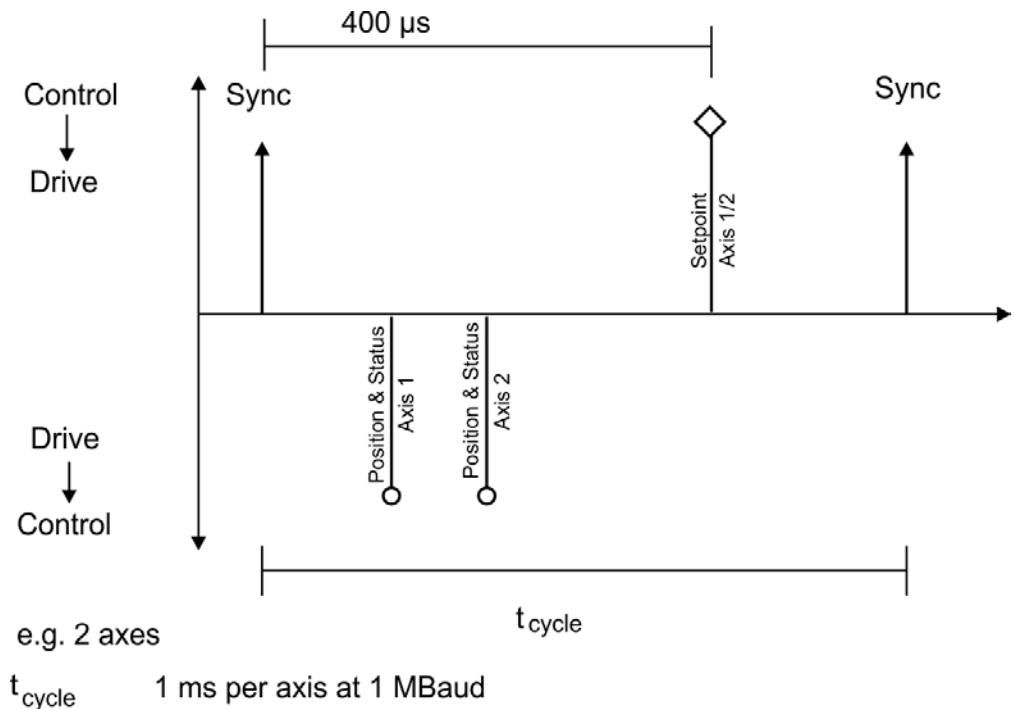
R PDO 2 can now be used to supply trajectory data for both axes, e.g.:
