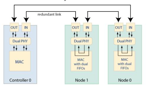
A SyngNet Ring with a controller and two nodes
