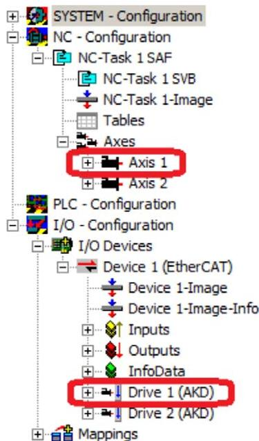
In order to connect to the drives using WorkBench, the drives must be either in Pre-Op, Safe-Op or Op state. State machine for a drive can be accessed from the Online tab for the corresponding drive under the I/O Configuration → I/O Devices → Device [x] → Drive [x] node (see screenshot below).
