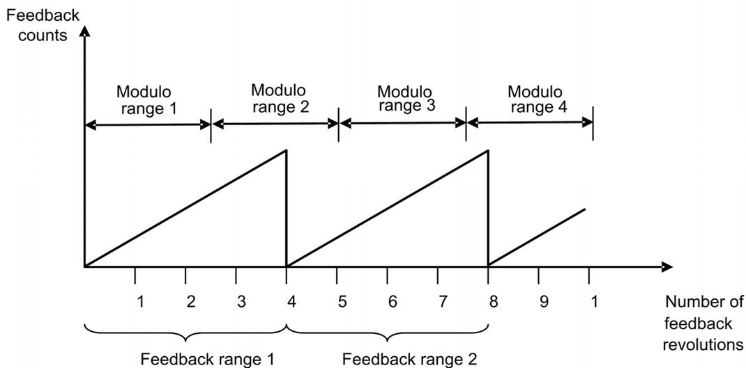
As described in the figure above, the selected modulo range is not repeated exactly at the place where the connected multiturn feedback rolls over. The application can move for several multiturn feedback ranges, but the drive cannot calculate the modulo position correctly after a power cycle.
