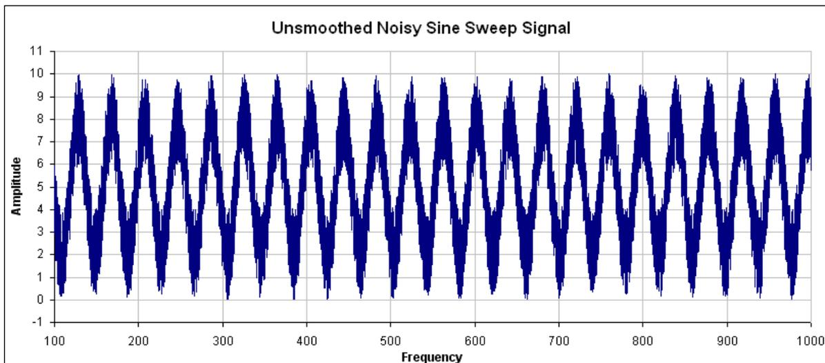
In this example, examining how the smoothing filter affects a single point shows how the smoothing filter works on a full plot. If you zoom in on 200 Hz +/- 5%, this gives a range of 190 Hz – 210Hz. The smoothing filter
