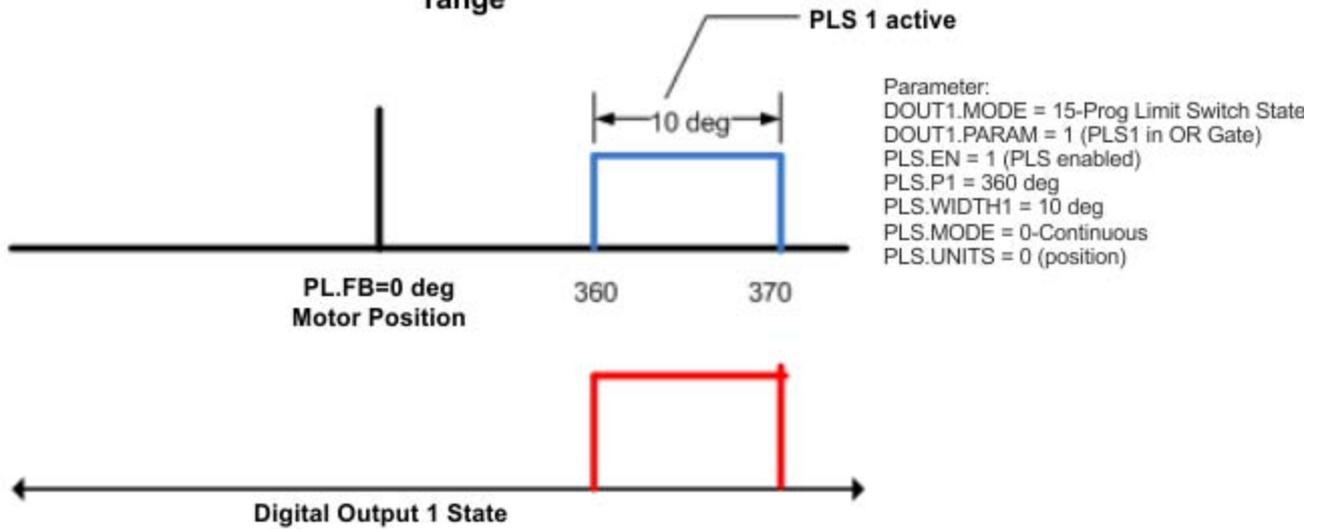
To setup an output with multiple turn-on points, configure and enable more PLS's and include them in the OR Gate.
