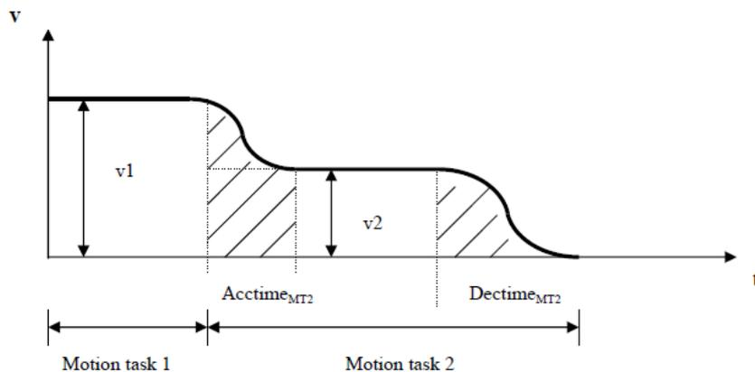
In case that the distance to the target position of the motion task 2 is smaller than  $distmin$ , the AKD generates a profile as shown in the next figure.
