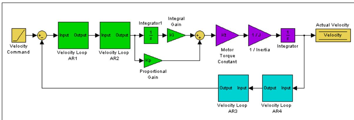
These blocks can be grouped into Controller, Plant, and Feedback sections:
