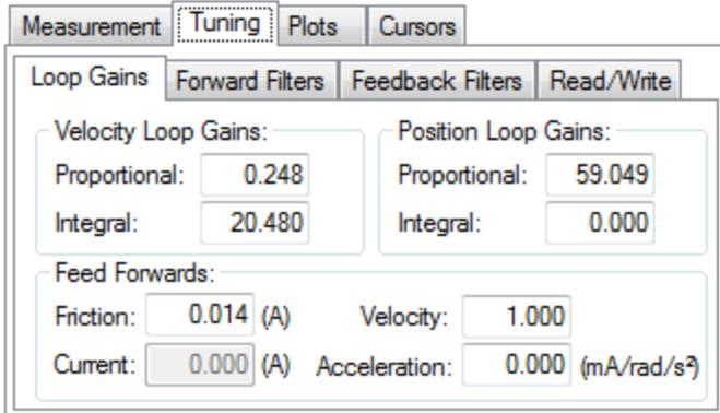
This tuning interface loads the tuning parameters on the drive each time a measurement is taken. Tuning parameters are split up into Loop Gains (Velocity Loop, Position Loop), Forward Path Biquad Filters, and Feedback Path Biquad Filters.
