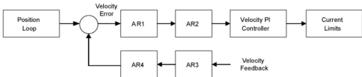
AR1, AR2, AR3, and AR4 are used in velocity and position mode, but are disabled in torque mode.
