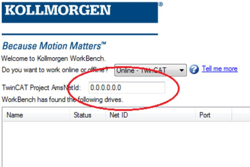
The project AmsNetId can be found in the TwinCAT System Manager under the NetId Management tab in Route Settings. Enter this Id number into WorkBench to discover the drive.
