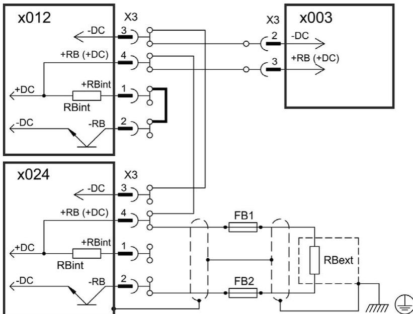
Without DC Bus fuses, other devices can become damaged or destroyed if, for example, a device fails due to an internal short circuit. If multiple drives are connected in parallel, then it is usual to insert DC Bus fuses ( ) between groups of drives (with a group consisting of two or three devices, depending on the current) in order to limit any possible resulting damage. Fuses cannot avoid damage by current peaks completely.
