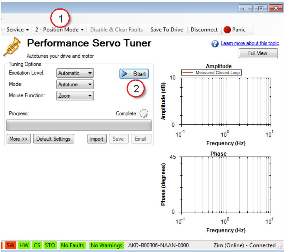
The PST will then perform several tests and display results as shown below. The progress bar (1) shows the relative progress of the PST, so you can estimate when the tuning will be finished. When the tuning is complete, the green **Complete** LED (2) illuminates, and a Bode plot (3) is displayed showing the frequency response of the tuned system.
