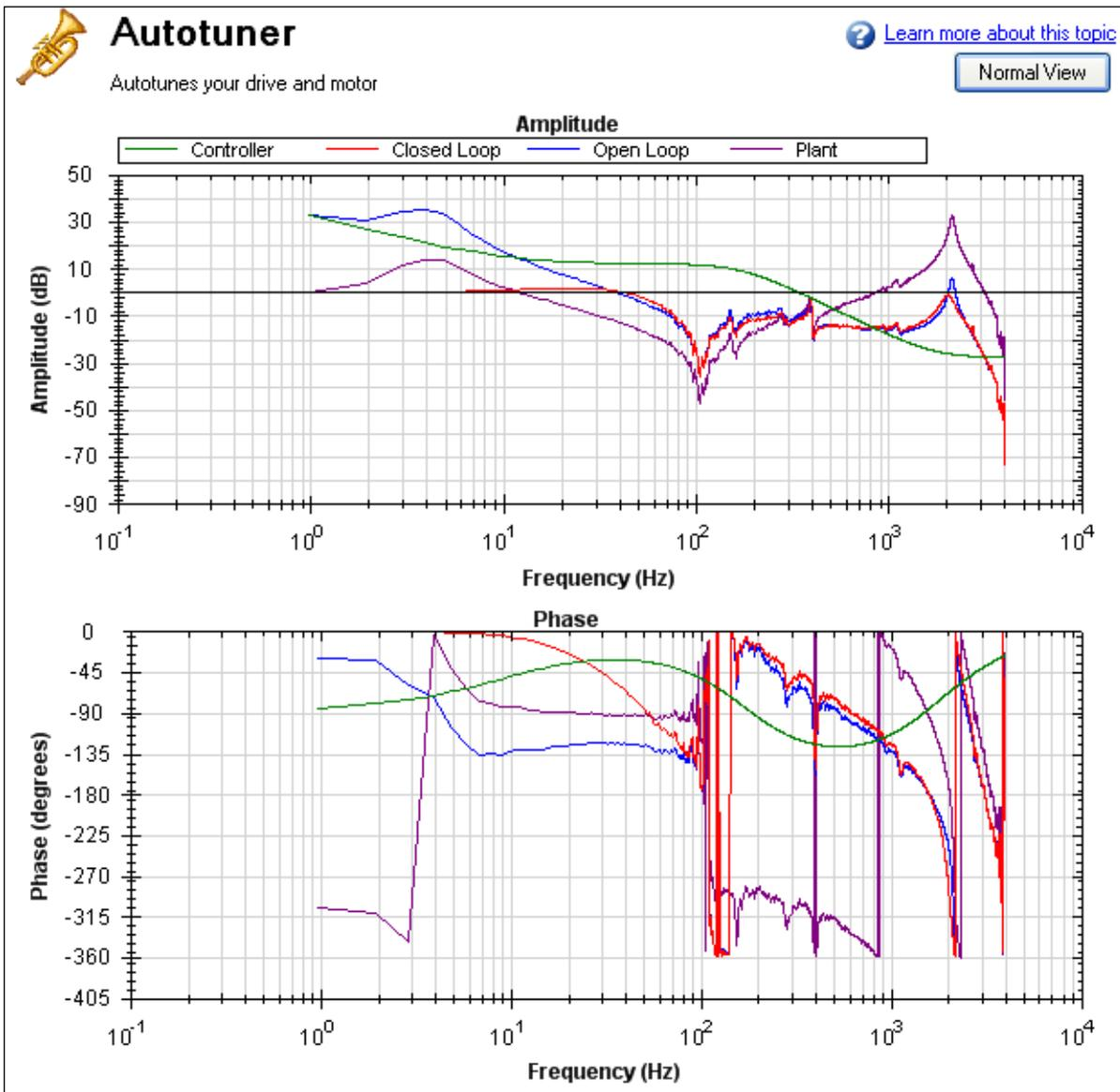
One way to resolve this problem is to use a low-pass filter in the feedback path. To use this filter, simply check the **Enable Lowpass Search** in the PST, which is the default behavior.
