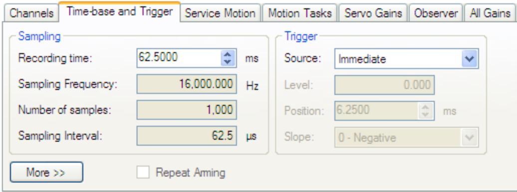
In this tab, you can set length of recording in ms and the sampling frequency in Hz. The number of samples is a calculated value displayed for reference. You can also choose the trigger source to be **Immediate** (triggers as soon as you click the **Start Recording** button) or to be one of many predefined sources.
