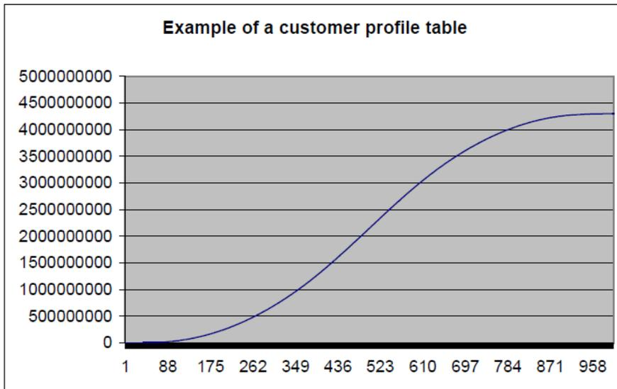
The motion profile table is the integral of the velocity profile. The velocity profile during the acceleration and the deceleration process is shown below:
