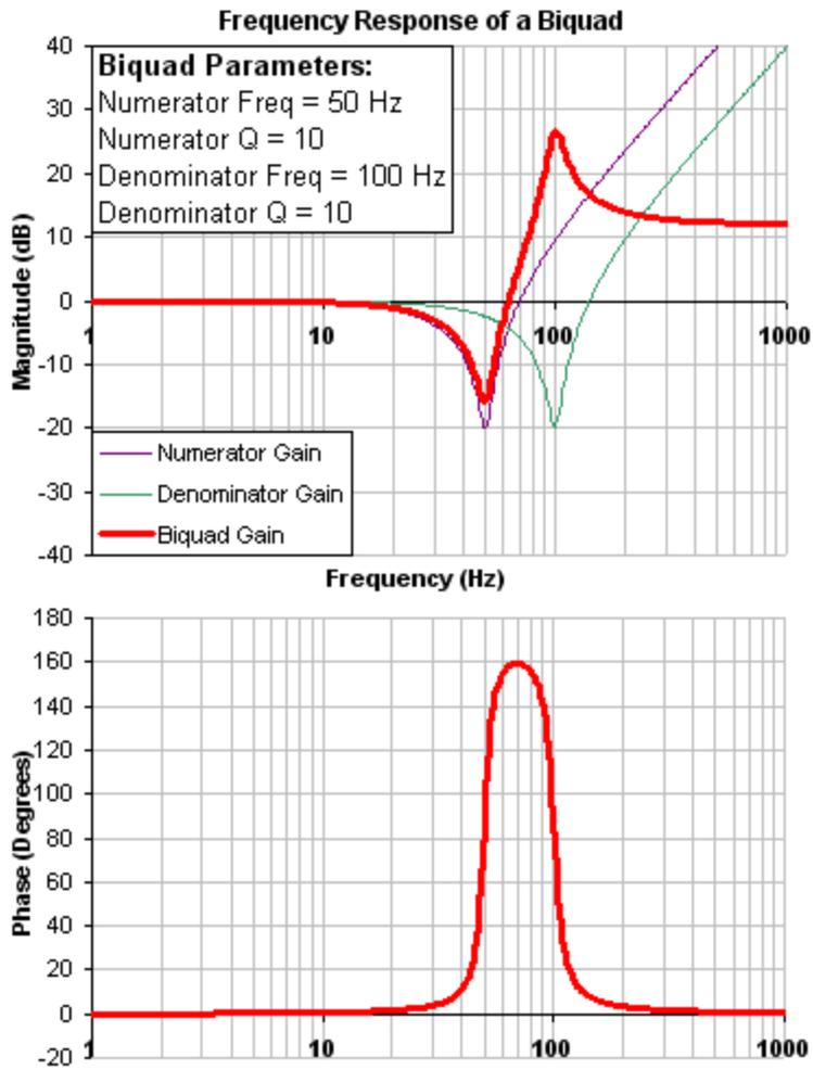
The previous two examples used a numerator frequency lower than the denominator frequency, yielding a positive gain in high frequencies. If the denominator frequency is lower than the numerator frequency, then high frequencies will have a negative gain.
