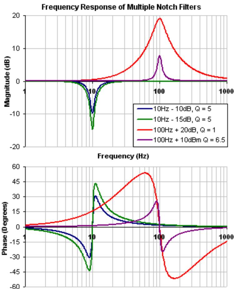
To specify a notch filter, you must specify the Frequency (Hz), Depth (dB) and Width (Q) of the notch. To do this, see the following example by clicking on the Velocity Loop:
