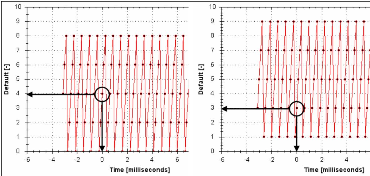
2. You can miss triggers, whose duration is less than N samples, where N is the value of REC.GAP. This is because the trigger is only evaluated every N samples.
