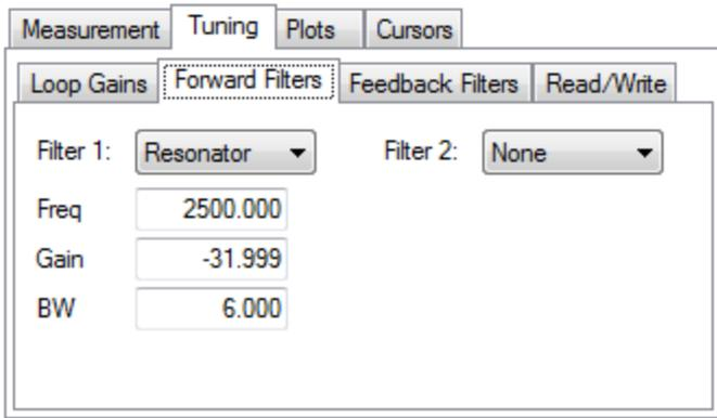
The resulting frequency response using the above resonator configuration is shown below:
