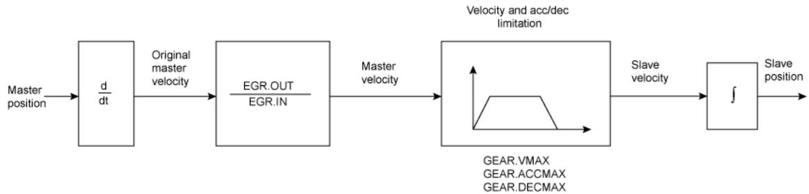
**Block diagram of the electronic gearing feature**
