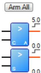
Setpoints can be armed using CMPx.ARM. In WorkBench, all setpoints can be armed for a given engine using the **Arm All** button. If a setpoint is armed, an A will appear in the bottom right corner of its graphic.
