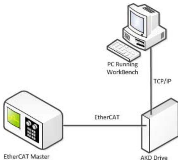
When the fieldbus is operational the AKD uses the FBUS.PROTECTION parameter to allow the user to select how commands from WorkBench, or any other device sending commands to the drive through a service channel, should be handled. WorkBench can use either of two service channels: Telnet or ASCII SDO. Both service channels are affected identically by FBUS.PROTECTION.
