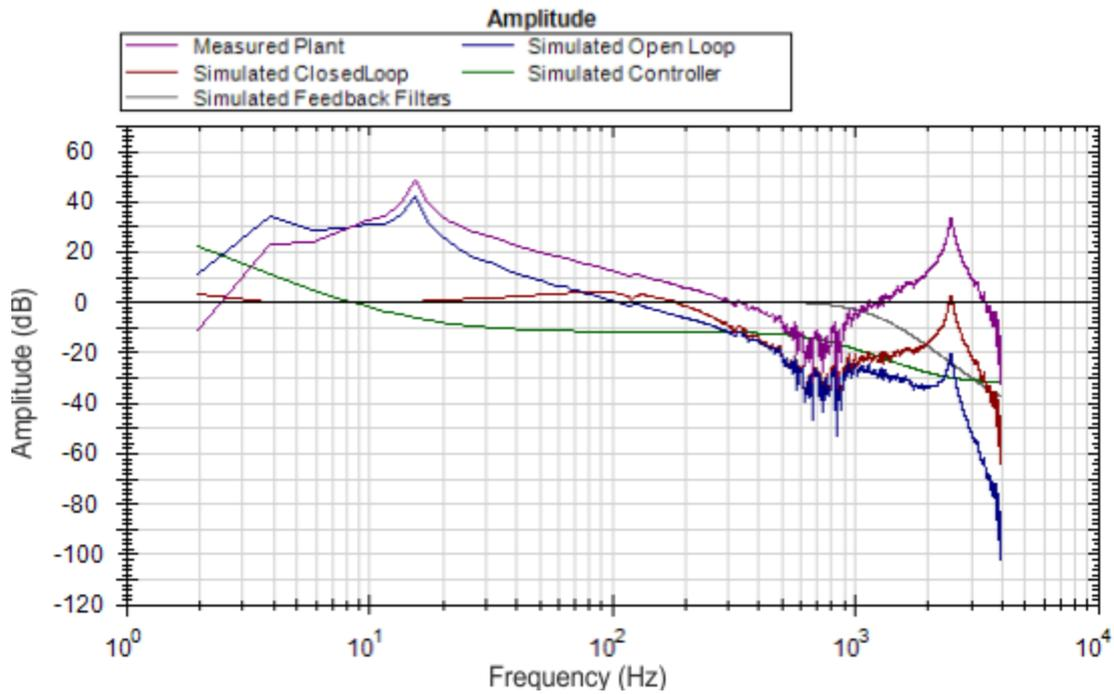
The Velocity Loop Proportional gain here is 0.248. If an application did not need to be tuned as stiff as this, then you could use the PST simulator to detune the motor to the desired bandwidth. A followup Bode Measurement can verify that the simulated response is correct.
