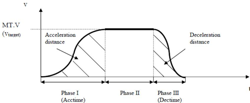
The drive calculates the acceleration time and deceleration time out of the given motion task parameters (see MT Parameters and Commands (→ p. 1035)) with the assumption of a trapezoidal acceleration setting (MT.ACC (→ p. 1036) and MT.DEC (→ p. 1045)). The formulas are:
