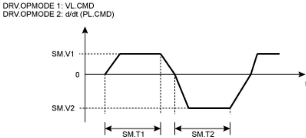
The deceleration process from SM.V1 or SM.V2 to 0 is not included in SM.T1 and SM.T2, respectively. SM.T1 and SM.T2 start as soon as the command value has reached the velocity 0.
