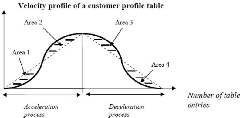
The left half of the curve describes the shape of the acceleration process of the motion task. The right half of the curve describes the shape of the deceleration process of the motion task. A symmetric motion profile table means that Area 1, Area 2, Area 3 and Area 4 have the same size.
