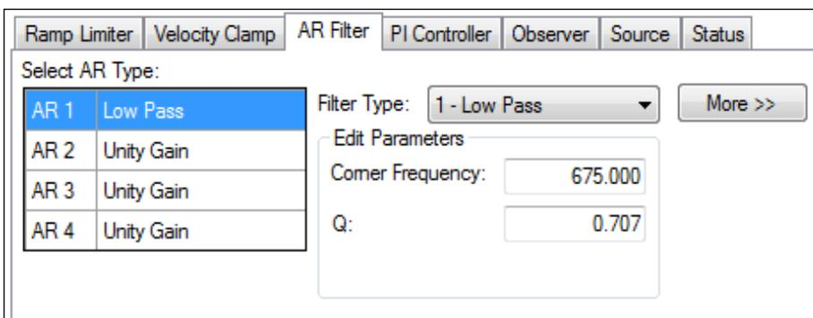
The default value for the low-pass filter is 675Hz. The low-pass filter is important for disturbance rejection, and it also reduces the audible noise of the system.
