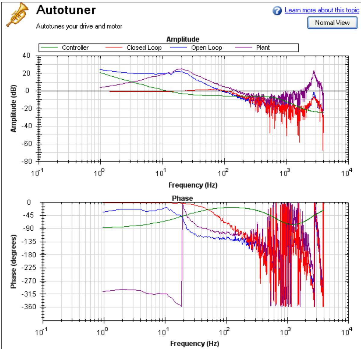
To make the Bode plot easier to read, increase the smoothing factor (1) in the advanced **Measurement Options**.
