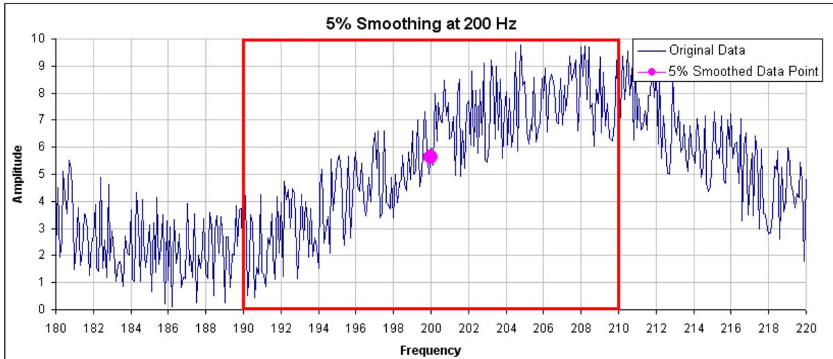
In the PST, the smoothing filter will do this analysis for every frequency point on the Bode plot. If the data is too noisy, then you can increase the smoothing percentage to smooth the noise out and see the underlying data patterns. A comparison of a system with 0.1% smoothing and 8% smoothing is shown below.
