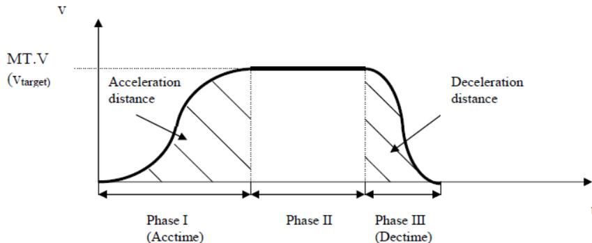
The Profile Table interpolation for a stand-alone motion task (the motion task does not automatically trigger a following motion task) can be separated in three different phases:
