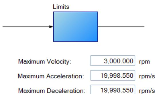
These limits (GEAR.ACCMAX, GEAR.DECMAX, GEAR.VELMAX) are applied only during gearing mode and the units are consistent with speed and acceleration of the output motor. All other limits in the drive are active along with gearing limits.
