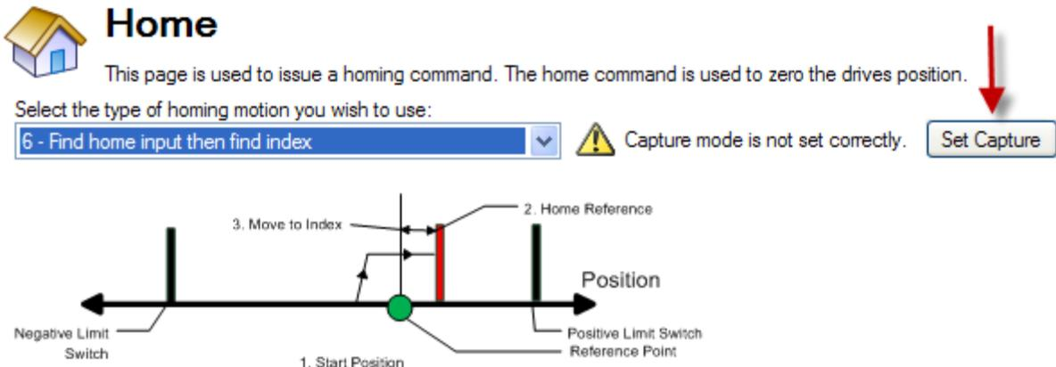
The home-switch must be activated according to the setting of the HOME.DIR setting.
