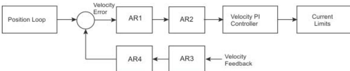
AR1, AR2, AR3 and AR4 are used in velocity and position mode, but are disabled in torque mode.
