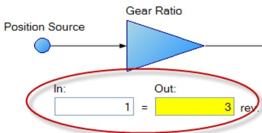
The position command (DRV.HANDWHEEL) reads the EEO value, where 4,294,967,296 is a full revolution of the input, then the value rolls over. Gear ratio does not affect the EEO value. If the output is set to 3 output revs per input rev, there will be 4,294,967,296 counts per 3 revolutions of the motor.
