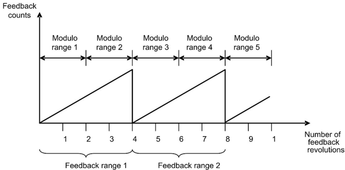
As described in the figure above, the selected modulo range of the drive is repeated exactly at the point where the connected multiturn feedback rolls over (Modulo range 1, 3, 5...). The application can move for several multiturn feedback ranges and the drive can recalculate the modulo position correctly after a power cycle. The positions within the modulo ranges represent the same value in modulo format for each feedback range.
