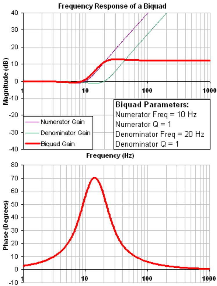
The biquad filter is very flexible, which allows custom filters to be designed. Below is an example of a resonance filter using a biquad. Notice how the high Q values affect the numerator and denominator. This gives a biquad frequency response similar to a mechanical resonance.
