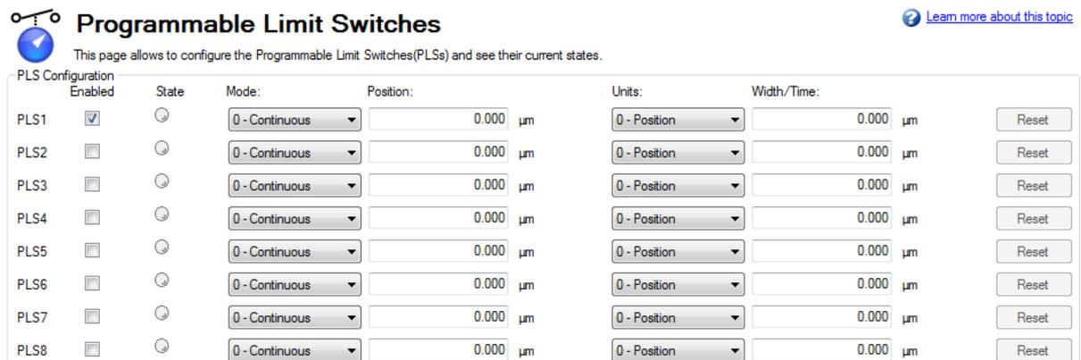
The PLS configuration section of the screen sets the mode and limits of each of the eight PLSs. The PLS is ignored unless it is enabled (see image above). In the screen example, PLS1 is set for continuous operation in position mode. Every time the 360 degree position (PL.FB) is crossed in either direction, the output will turn on for 10 degrees of motor movement.
