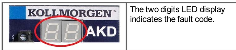
The additional runtime fault messages for AKD-T are coded with numbers starting from F801. All faults activate the fault relay and can be cleared with `DRV.CLRFAULTS`.
