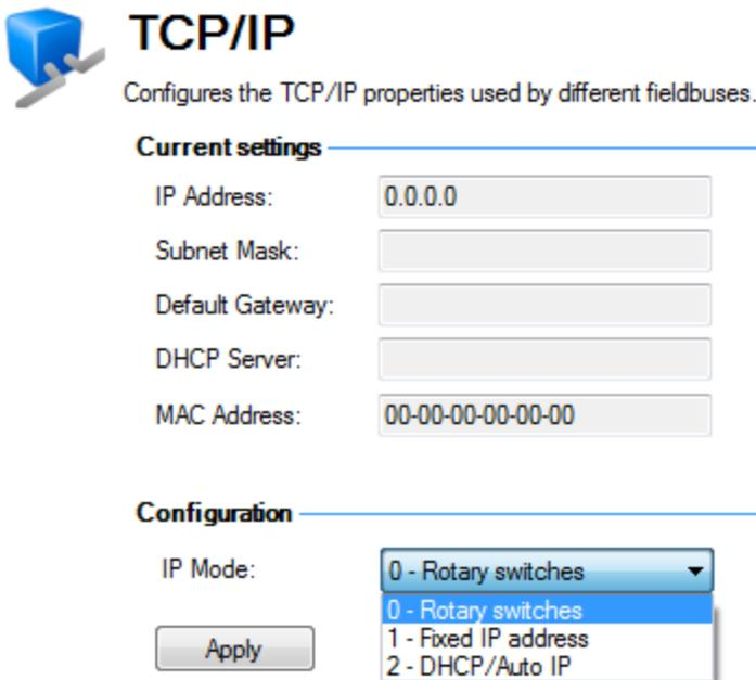
There are three modes under IP Mode on the TCP/IP screen by which the IP address can be set.
