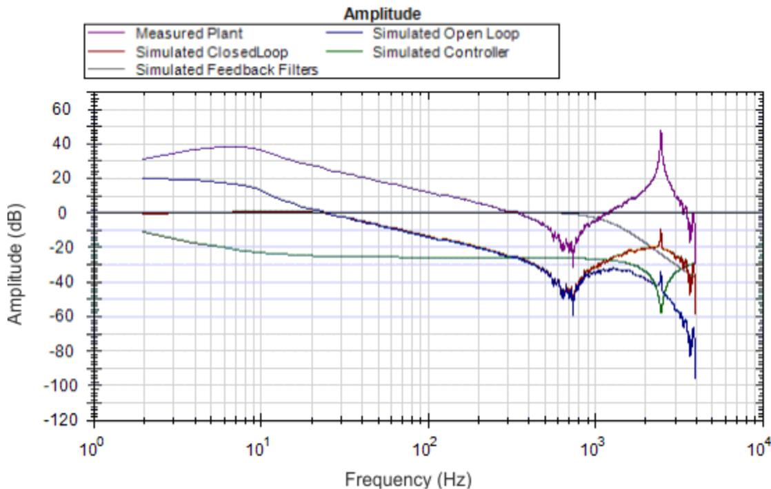
Notice the attenuation of the resonance in the blue and red traces (open loop and closed loop, respectively).
