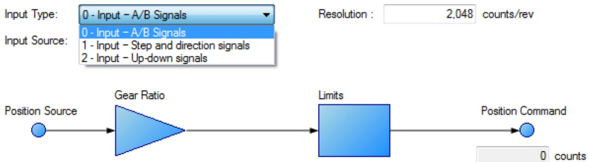
Resolution is the post-quadrature value of the counts/revolution of the input. Additionally, a gear ratio can be applied to affect the output ratio of the motor.
