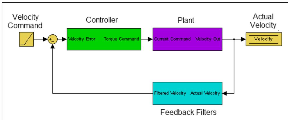
All of the green blocks have been grouped together to create the Controller [C]. The Controller is the portion of the control loop containing all velocity and position loop tuning, including the forward path filters.
