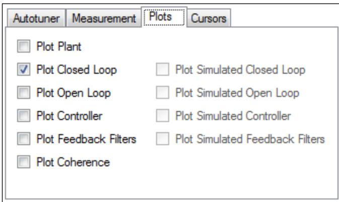
By default, only the measured closed loop plot is selected. You can control which of these responses are displayed on the Bode plot by checking or unchecking the **Plot Plant**, **Plot ClosedLoop**, **Plot Open Loop**, **Plot Controller**, and **Plot Coherence** checkboxes shown. The options **Plot Simulated Closed Loop**, **Plot Simulated Open Loop**, **Plot Simulated Controller**, and **Plot Simulated Feedback Filters** are only available in Bode plot mode, not PST mode.
