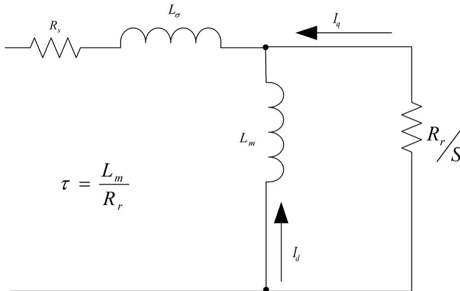
Alternatively, the rotor time constant can be estimated from the rated current, magnetizing current (MOTOR.IMID (→ p. 980)) and rated slip frequency as follows:
