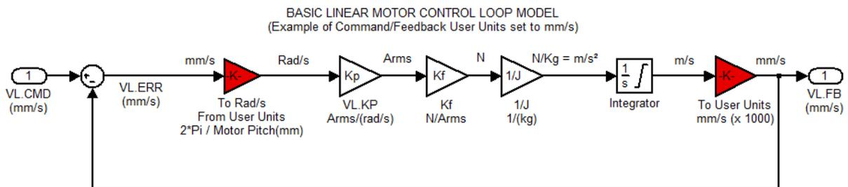
The red blocks are automatically handled at the drive level.
