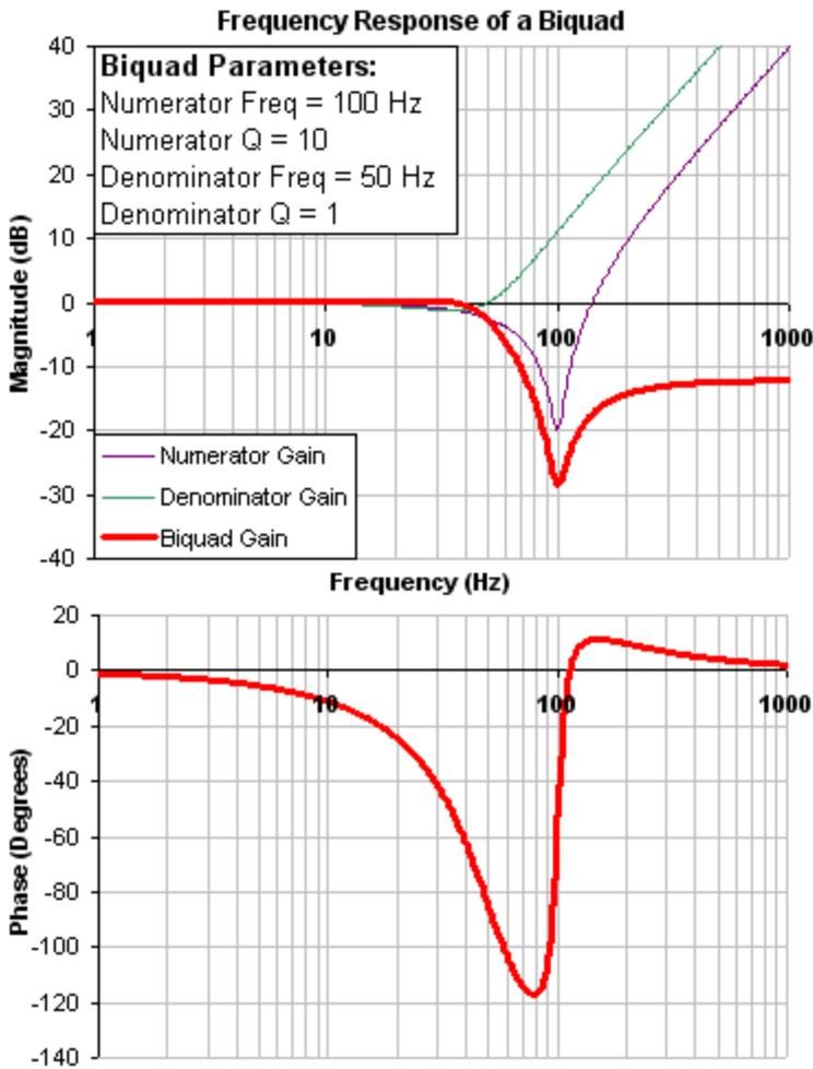
To specify a biquad filter, you must specify the frequency and Q for both the zero and the pole on anti-resonance filter 3. To do this, see the following example using the terminal commands that sets:
