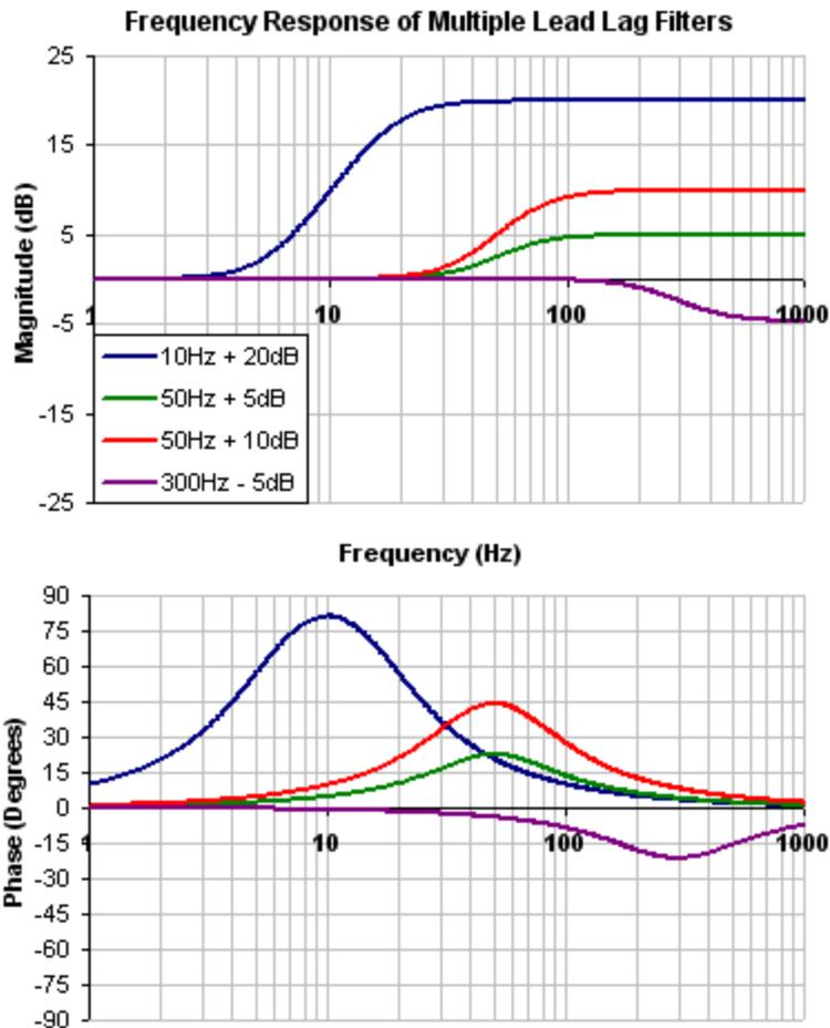
To specify a Lead Lag filter, you must specify the Center Frequency and high frequency Gain (dB). To do this, see the following example by clicking on the Velocity Loop:
