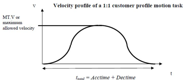
Note that the motion task target velocity is only reached in case of a symmetric table. The velocity will be different when the profile table is non-symmetric.
