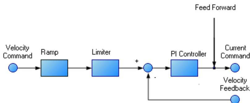
Procedure for simple velocity loop tuning:
