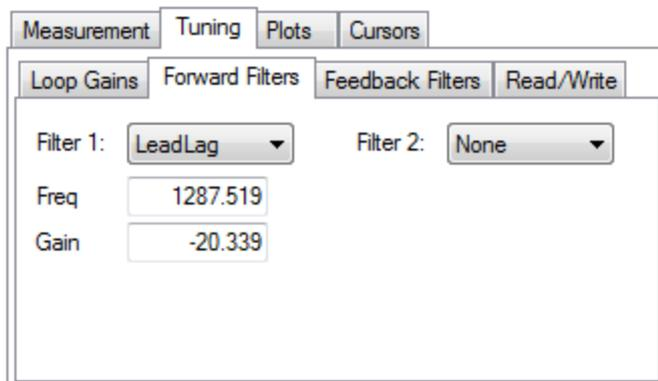
The results of the autotune are still on the drive, and provide adequate tuning. A lead lag filter is the default tuning filter, and is a good general case filter for most servo loops.
