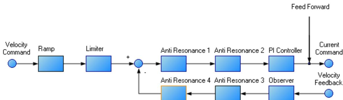
To perform basic tuning of the velocity loop, you can use just the PI block and set ARF1 and ARF2 to unity (no effect) and set the observer to 0 (no effect). Using just the PI block simplifies the process of tuning the velocity loop. To start tuning you can adjust the PI Controller block first. A simplified velocity loop without anti-resonant filters and observer is shown below. This is how you can think of the loop before the anti-resonant filters and observer is used.
