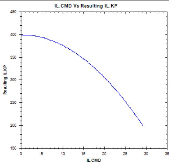
By default, the current loop value will be what is defined in IL.KP across the whole range of currents. To change the value of IL.KP over a range of values, simply enter a scaling term: 0 - 100% of the current value.
