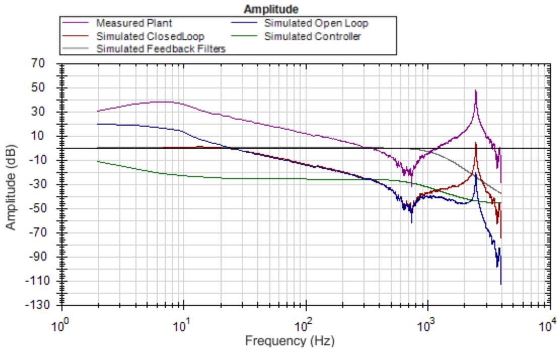
The new measured Bode Plot indicates we achieved slightly lower than 30 Hz bandwidth. The servo is stable, and tuning can be refined until desired performance is reached.
