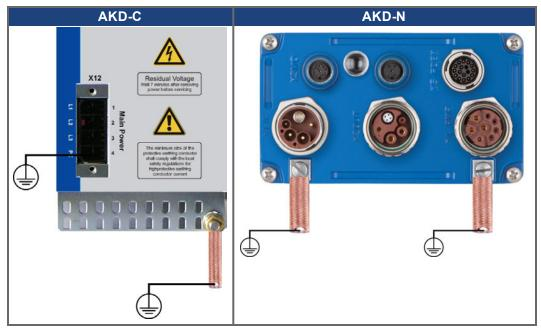
The leakage current against PE is more than 3.5 mA. In accordance with EN 61800-5-1, the PE connection must therefore either be double implemented or a connection cable with >10mm² cross-section used.
