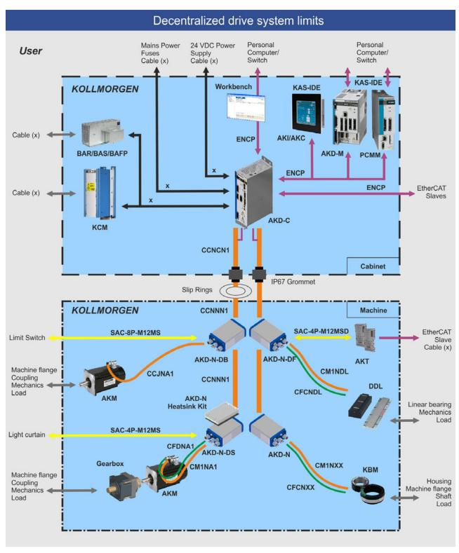
All components in the blue rectangle are products delivered by Kollmorgen. Elements in the gray area show, and the cables signed with "x" are components which have to be added by the machine builder.
