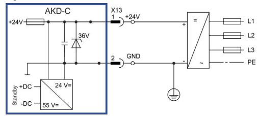
The 24V supply input of the AKD-C is short circuit-proof. Secure the 24 V power supply units used in accordance with the supply line cross-sections used.
