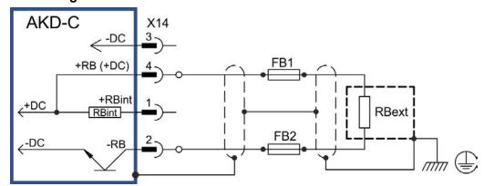
The fuses do not protect the brake resistor from thermal overload. this supervision is done by the amplifier's software, if the parameterizing is correct. The fuses shall protect from short circuit and earth short circuit!
