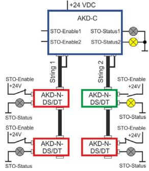
Torque Drive 1 in String 2 safely locked.
