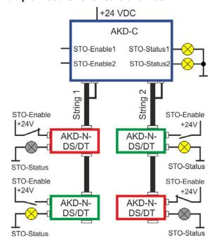
Torque Drive 2 in String 1 safely locked.
