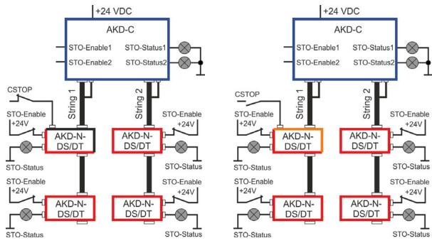
Torque for all drives released. Drive 1 in String 1 produces torque, CSTOP is not active.
