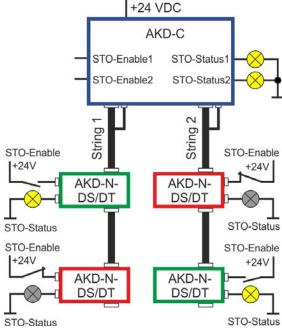
Torque Drive 1 in String 1 safely locked. Torque Drive 2 in String 2 safely locked.
