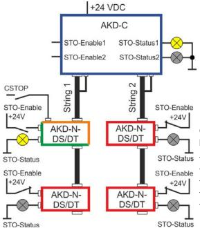
CSTOP for drive 1 in String 1 is activated, torque is safely locked. Torque for all other drives is released.
