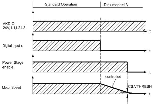
If velocity drops below threshold CS. VTHRESH or timeout occurs brake is applied.
