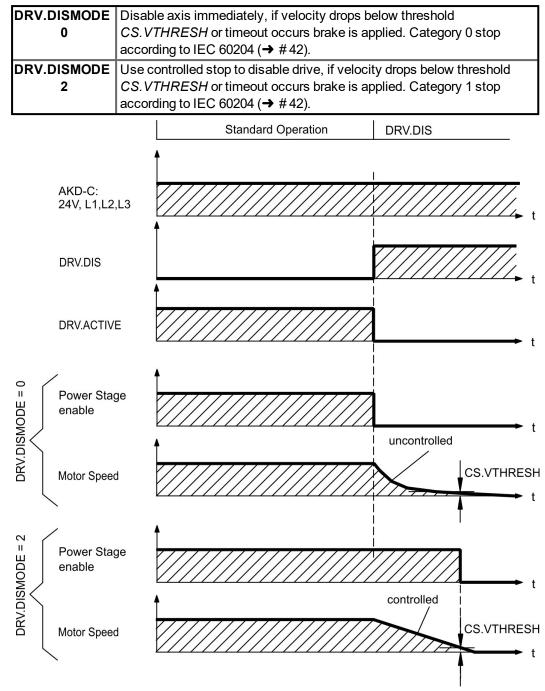
If velocity drops below threshold CS.VTHRESH or timeout occurs brake is applied.
