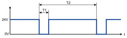
Test pulses with T1 < 300  $\mu$ s and T2 > 200 ms will not have any influence to the safety relevant STO function. Test pulses, which are outside of this specification, will switch the STO function, but will not create a dangerous situation.
