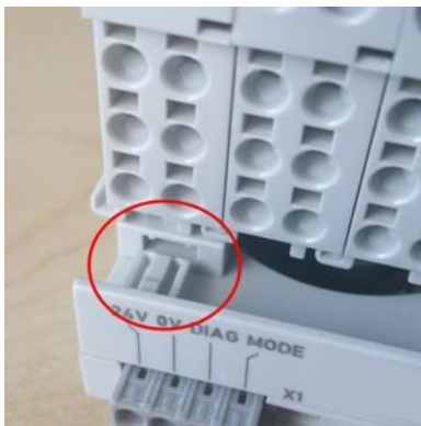
Figure 3-6: Push latching tab into groove
