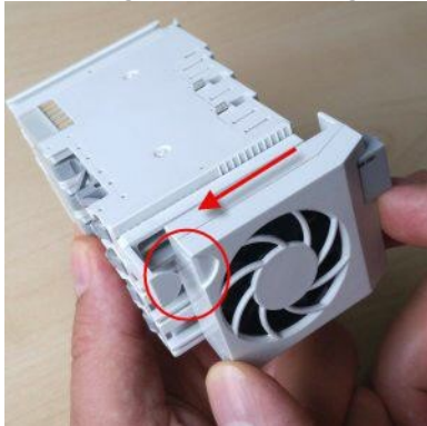
Attaching the fan cartridge
