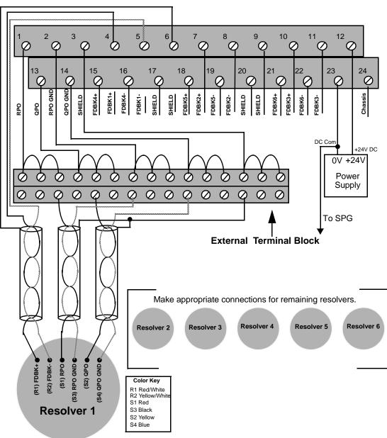
**Block Input Resolver Module Screw Terminals**
