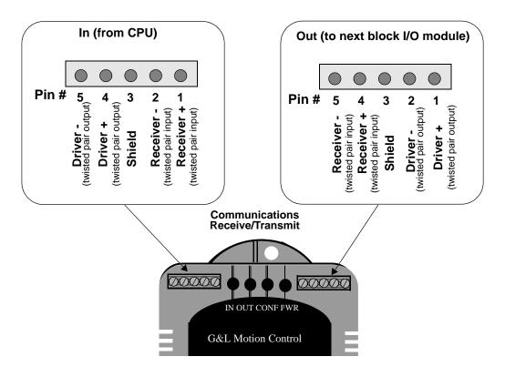
Figure 13-3 Pinouts for Communication Connectors
