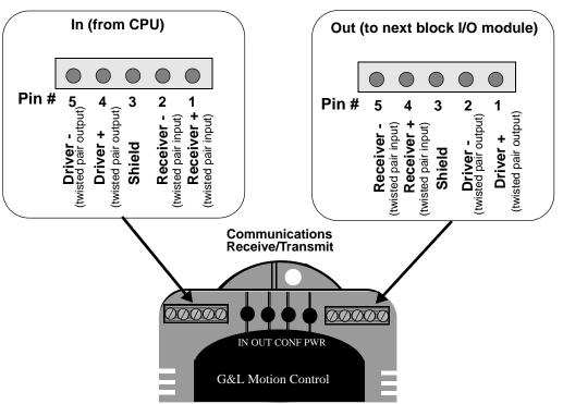
Figure 3-4 Pinouts for Communication Connectors
