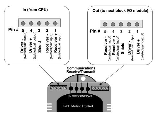
Figure 7-8 Pinouts for Communication Connectors
