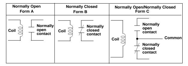
Figure 7-9 Relay Forms A, B, and C
