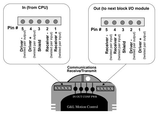
Figure 11-7 Pinouts for Communication Connectors
