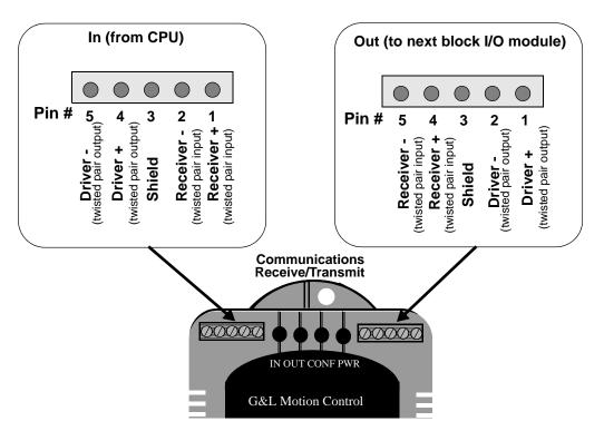
Figure 10-10 Pinouts for Communication Connectors
