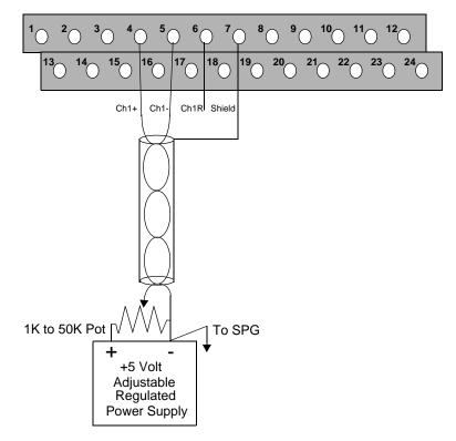
Figure 11-6 Adding an External Potentiometer
