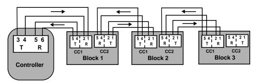
**NOTE:** CC represents the communication connections at the top of the block modules.
