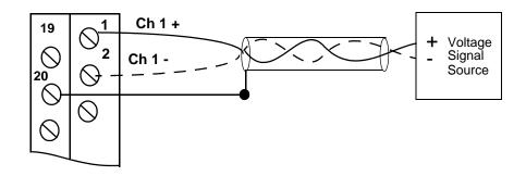
If the  $\pm 100$  mV range will be exceeded, external resistors must be added. The resistors should be positioned as close to the Block I/O module as possible.
