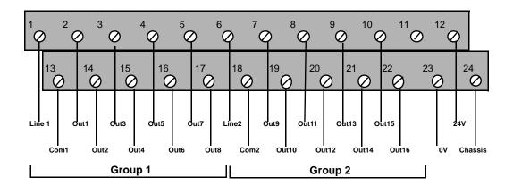
Figure 3-2 Screw Terminal Connection Assignments
