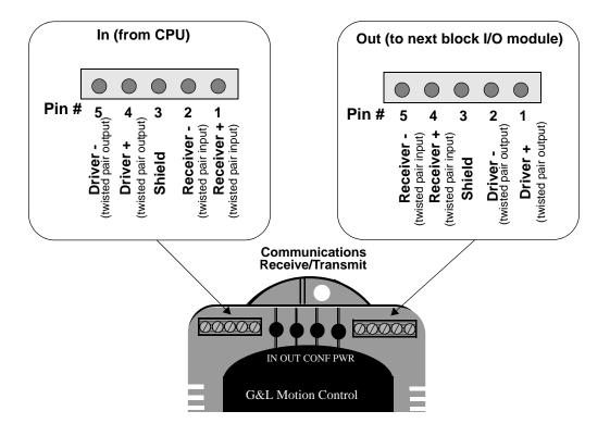
Figure 8-4 Pinouts for Communication Connectors
