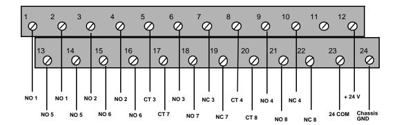
Figure 7-2 Screw Terminal Connector Assignments
