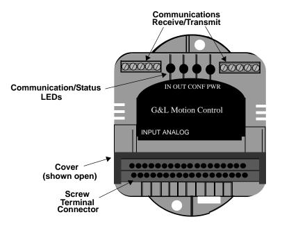
Figure 11-1 Block Input Analog Module (4 Channel)
