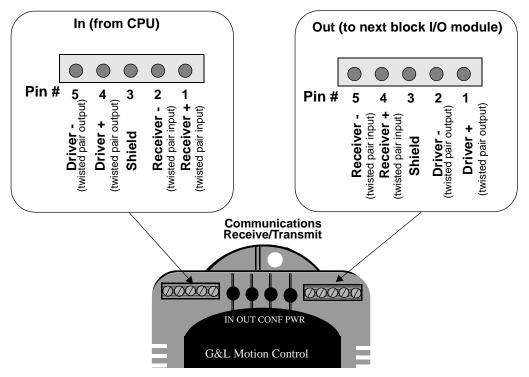
Figure 14-4 Pinouts for Communication Connectors
