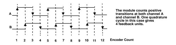
For each encoder channel, there is a 24-bit up/down counter. It is incremented or decremented in accordance with the signals received from the differential quadrature encoder. There is also a 24-bit latch associated with each encoder input channel.
