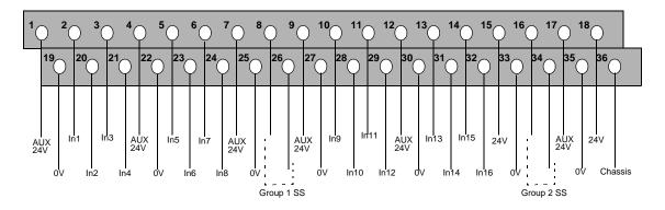
Figure 14-2 Screw Terminal Connector Assignments
