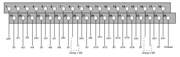
Figure 4-2 Screw Terminal Connector Assignments
