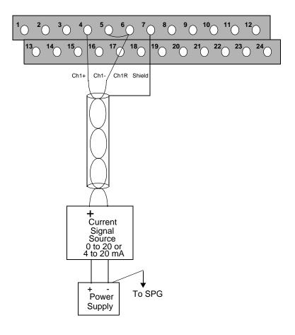
An alternative method of connecting a two wire 4 to 20 mA current device is shown in Figure 11-5. Place a jumper between the - input and the  $250\Omega$  resistor input.
