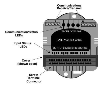
Figure 14-1 Block Input 24V DC Module/J 16 point
