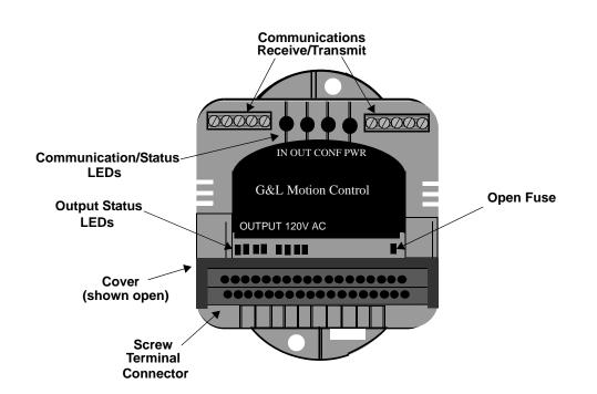
Figure 6-1. Block Output 120V AC Source Module (8 points)
