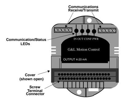
Figure 12-1 Block Output 4-20mA Module (4 Channel)
