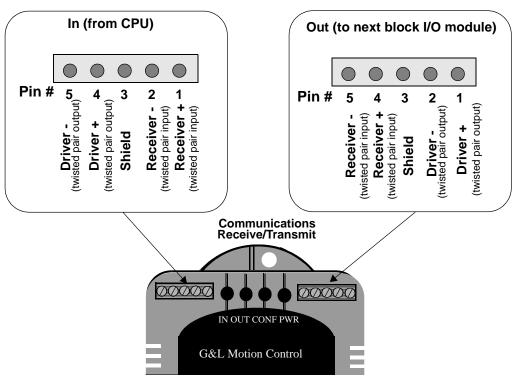
Figure 4-4 Pinouts for Communication Connectors
