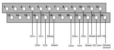
Figure 13-2 Screw Terminal Connector Assignments
