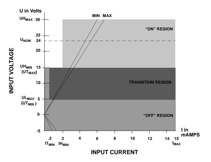
Figure 5-7 Input Characteristics Compared to IEC Standards
