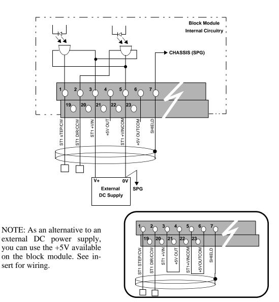
Figure 10-3 Connections for One Stepper Output
