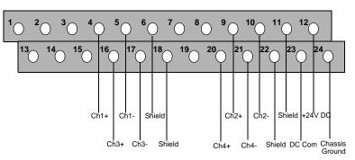
Figure 12-2 Screw Terminal Connector Assignments
