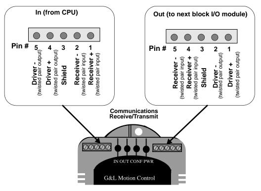
Figure 6-3. Pinouts for Communication Connectors
