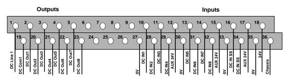
Figure 15-2 Screw Terminal Connection Assignments
