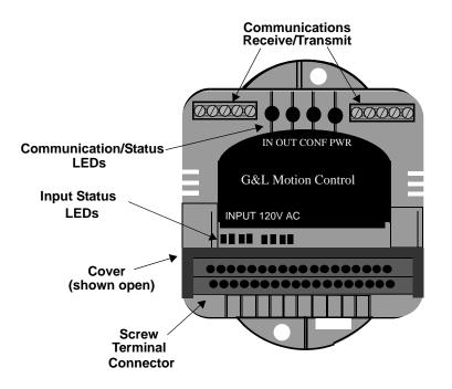
Figure 8-1 Block Input 120V AC Module (8 Point)
