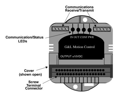
Figure 13-1 Block Output ±10V DC Module (4 Ch)
