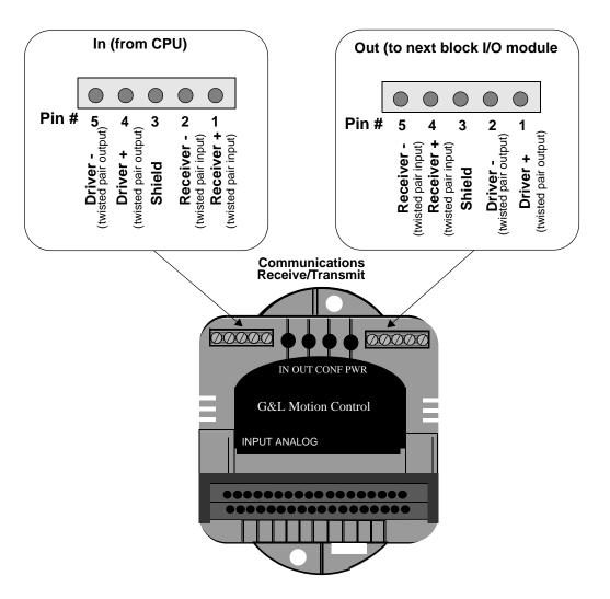
Figure 12-4 Pinouts for Communication Connectors
