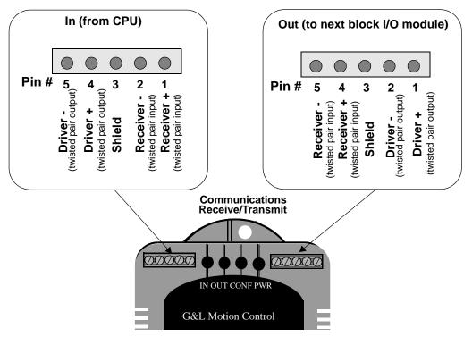
Figure 17-6 Pinouts for Communication Connectors
