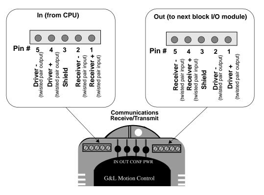
Figure 9-5 Pinouts for Communication Connectors
