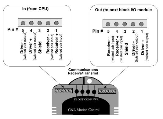
Figure 16-8 Pinouts for Communication Connectors
