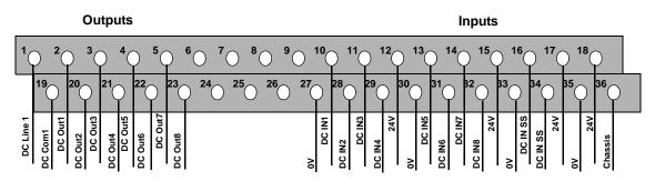
Figure 5-2 Screw Terminal Connection Assignments
