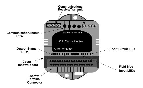
Figure 15-1 Block 24V DC 8In/8 Out Module/J
