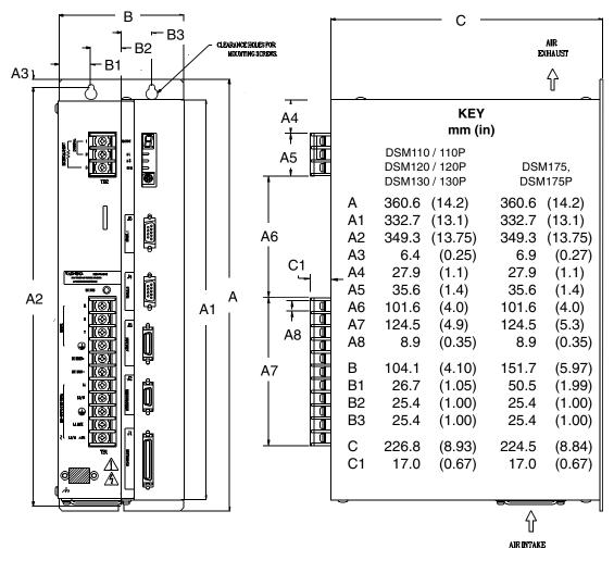
FIGURE 5.1 DSM Mounting Dimensions (sheet 1 of 2)
