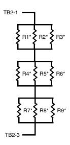
NOTES: A single resistor of equivalent total resistance may replace multiple resistors. Dissipation uses approximately 50% of total resistance value.
