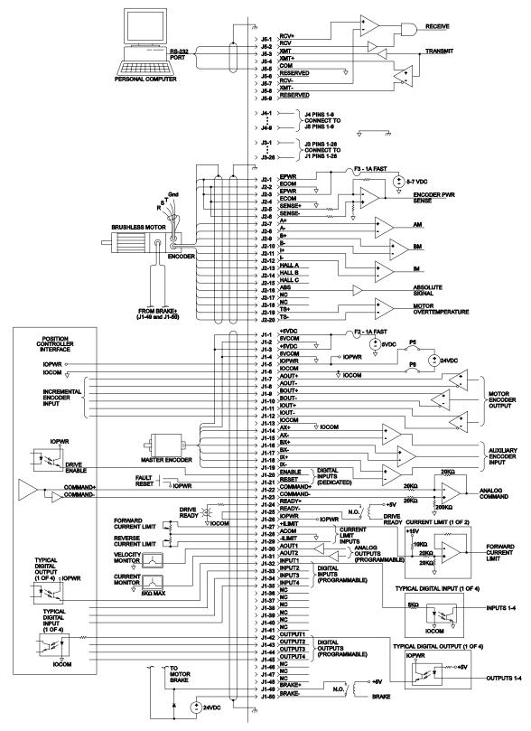
**DSM Interface Connection Diagram**
