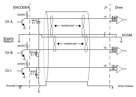
FIGURE 6.30 Single-Ended Encoder Interface via Open Collector Transistor with 24 VDC Pull-up (not recommended)
