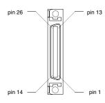
J3 is a 26 pin female mini-D ribbon connector (AMP 2-178238-4). It duplicates the first 26 pins of J1, the Controller connector, which are discussed in detail beginning on page 6-53. Contact between the connector shell and the grounded chassis provides shield termination.
