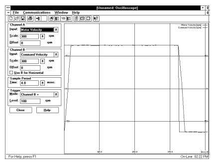
CRITICALLY DAMPED Motor Velocity quickly settles to the Velocity Command.
