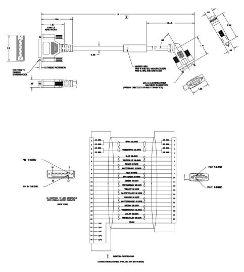
FIGURE B.7 J2 to 25-pin D-Connector Cable (supplied with kit 401-34408)
