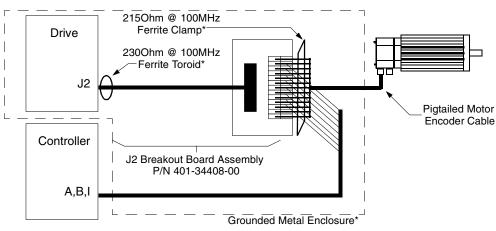
NOTE: An asterisk (\*) indicates an installation option to comply with EU EMC Directives. Either a grounded metal enclosure or ferrite cores provide the requisite EMC protection.
