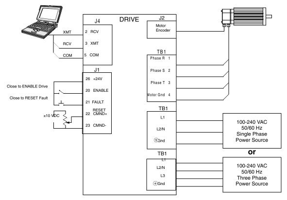
FIGURE 8.1 Analog Controller Connection Diagram
