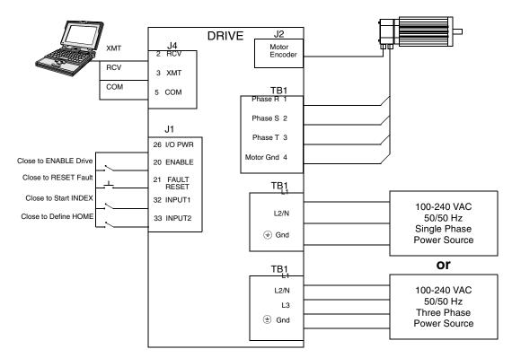
FIGURE 8.11 Absolute Indexing Connection Diagram
