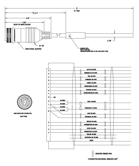
FIGURE B.11 FSM, HSM or SSM Series Motors to No Connector Encoder Cable (P/N 401-34425-XX)
