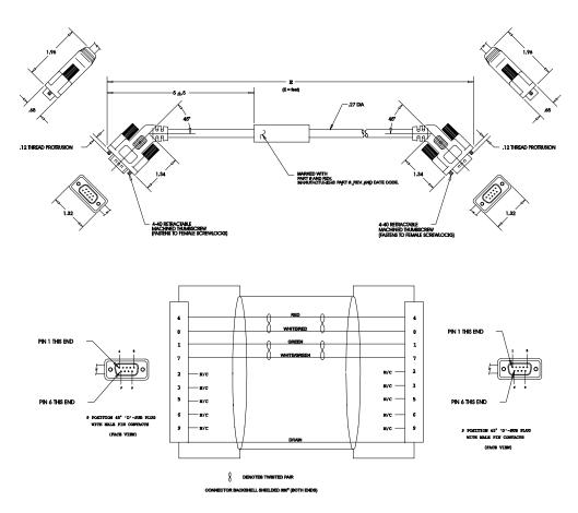
FIGURE B.9 J5 to J5 Serial Interface Cable (P/N 502-04021-XX)
