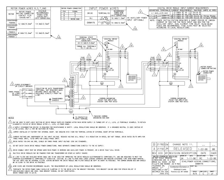
FIGURE 5.5 Power Wiring Diagram for DSM175 and DSM175P
