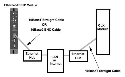
There are several different Client/Server configurations possible between the GLMC and CLX. When the GLMC is a Server it will respond to read/write requests from one or more CLX's which are the Client(s). The GLMC ladder will require two ASFB's to operate as the server. The E\_CIP\_CM ASFB is used to manage the TCP/IP Connection between the GLMC and one or more CLX's. The E\_CIP\_MR function is the Message Router for processing CIP over Ethernet requests from a CLX.
