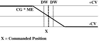
X = Commanded Position DW = Dead Band Window CV = Correction Velocity Max CG \* ME = Correction Velocity
