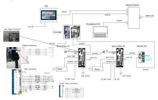
Figure 4-1: Connecting all the Hardware components
