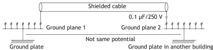
With longer distances, there is a risk that the ground potential may be different. In that case, the shield should only be connected at one end. A good alternative is to connect the other end of the shield to the ground via a 0.1 µF/250 V plastic capacitor. Both ends are then connected to the ground in terms of HF, but only connected to the ground at one end in terms of LF, thus avoiding the 50/60 Hz grounding loops.
