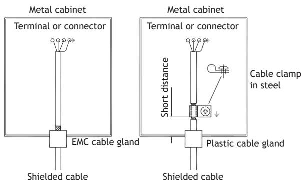
1. Use an EMC cable gland or regular plastic cable gland, remove the outer jacket and connect the shield to the installation plate with a 360° metal cable clamp.
