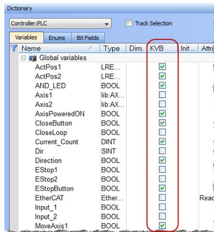
The Modbus tag addresses are defined automatically in the KAS IDE when the project is compiled, then transferred into KVB when the KVB project is opened from inside the IDE. Global or local variables can now be selected to share over Modbus. Each time the KAS IDE project is compiled the share list is updated.
