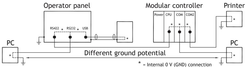
When a PC is connected to the HMI panel, the internal 0 V (GND) of the panel is connected to the protective ground via the PC.
