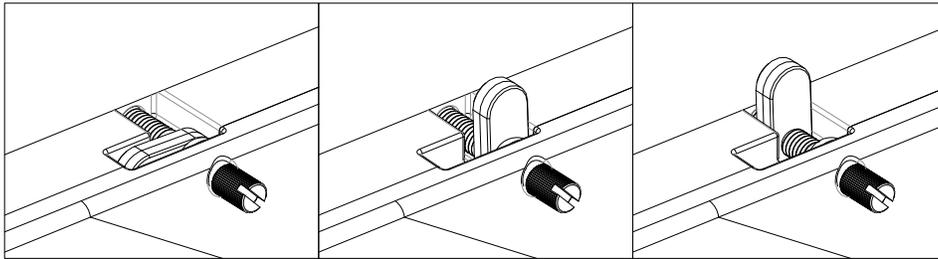
**Figure 3-1:** Tighten the screws to  $0.7 \text{ Nm} \pm 0.2 \text{ Nm}$ .
