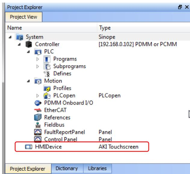
Double-clicking on it will also launch KVB. In this scenario tags and the target IP address are imported into KVB but the AKI Panel selection is not made in the IDE and must be configured in KVB:
