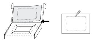
Secure the graphic operator terminal in position using all the fastening holes and the provided brackets and screws:
