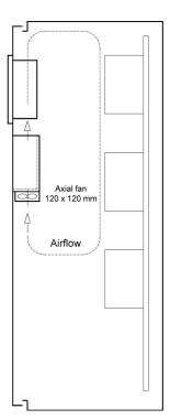
In most cases, the ambient temperature for the graphic operator terminal is significantly higher than the device cabinet's ambient temperature.
