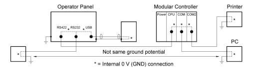
When a PC is connected to the terminal, the terminal's internal 0 V (GND) is connected to the protective ground via the PC.
