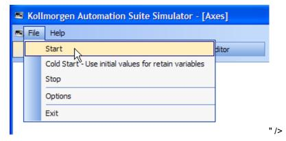
Figure 4-7: Start Device with the KAS Runtime
