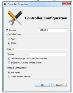
Figure 4-3: Configure the Controller Properties
