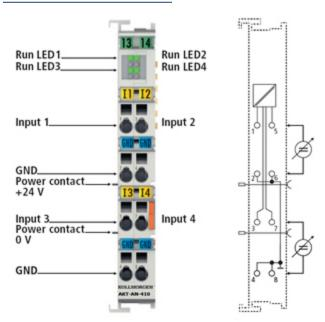
Top view, contact assembly, connection
