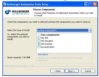
**Figure 3-2:** Install Run-time for Industrial PC (See the different Types of Deployment in paragraph "Installing KAS IDE" on page 10)
