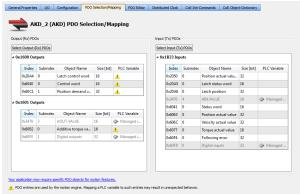
The PDO Editor tab allows you to modify PDOs which the device's manufacturer designated as editable.
