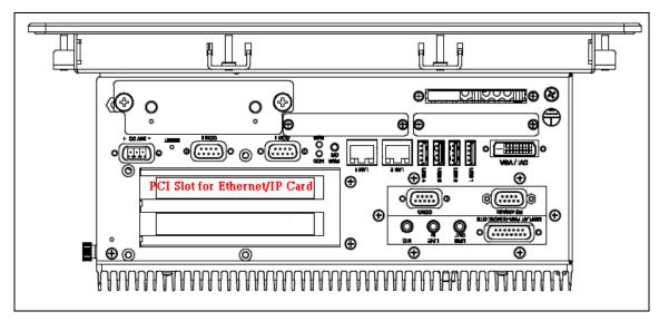
Figure 2.14: Ethernet/IP PCI Slot on a PAC with a Panel
