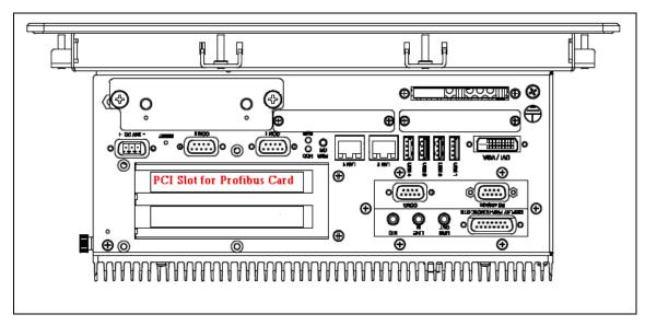
Figure 2.11: Profibus PCI Slot on a PAC with a Panel
