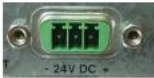
Figure 3.1 DC-connector (without Phoenix plug terminal)
