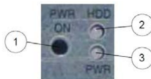
Figure 2.6 Power Button and LEDs
