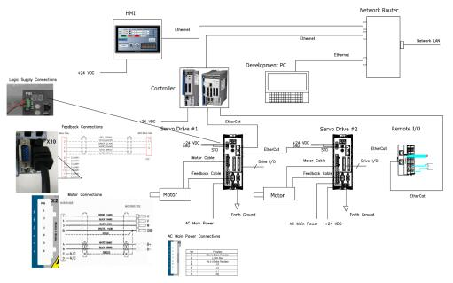
Figure 4-1: Connecting all the Hardware components
