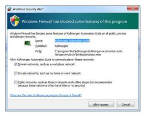
The Simulator uses port 80 for the web server. This communication channel is mandatory for Simulator to work properly. So please close any application, such as VOIP, that may use port 80 before starting Simulator.
