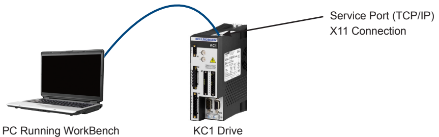
Figure 11 . Option A: Direct Connection
