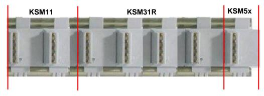
Power supply for KSM31R module is on the back plane bus and is generated from basic device. Supply for digital outputs is on X11 of KSM31R device.
