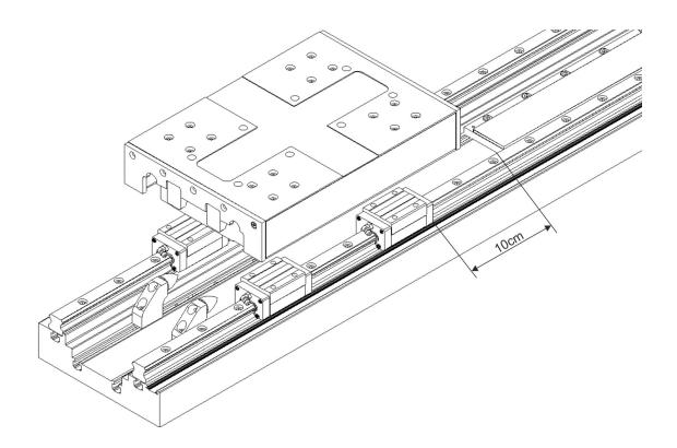
6. Carefully and slowly slide the linear motor assembly over the mounted magnetic plates and temporarily secure the motor against the mechanical end stop.
