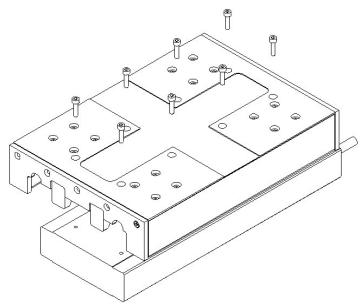
3. Mount and fix the first magnetic plate segment (the secondary part of the ICH linear motor) on the customized base with the fixing screws.
