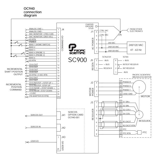
**Note:** Default functions for J4 connections are reprogrammed by the OC940. This configuration <u>does not</u> match the base SC900 configuration.
