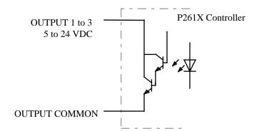
Typical output, current sinking to Output Common
