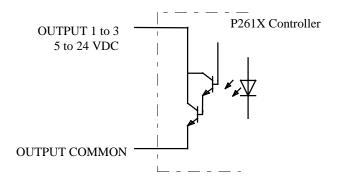
Typical output, current sinking to Output Common
