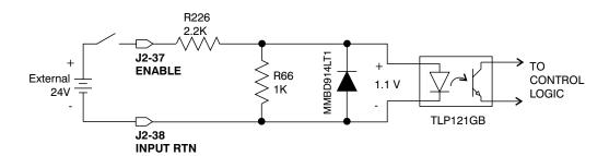
**Note:** If the drive's 24 V supply is being used, connect as shown below.
