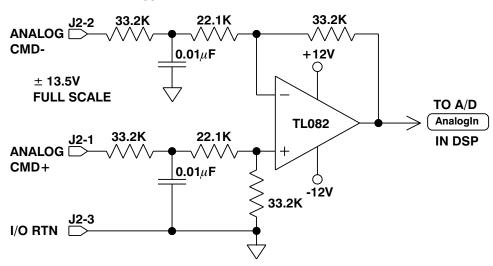
**Note:** Always connect I/O RTN (J2-3) to the signal ground of the source. Failure to do so may result in erratic operation.
