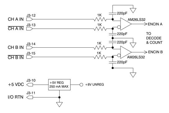
**Note:** An adapter can be powered from the serial port +5 Vdc output on J1-4 as long as the load current on J1-4, J2-14, and J3-10 total less than 250 mA.
