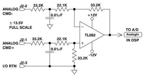
**Note:** Always connect I/O RTN (J2-3) to the signal ground of the source. Failure to do so may result in erratic operation.
