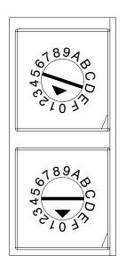
Note: The axis address is set to 1 by default at the factory.
